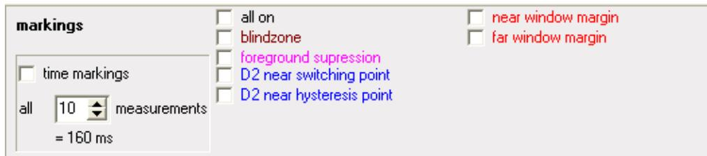
Blindzone, foreground suppression, switching- and hysteresis points (on sensors with switching output) and window margins (on sensors with analogue output)
