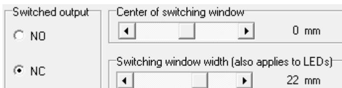
The switched output of the bks+../FIU or bks+../F can be used e.g. for monitoring purposes. He switches around the (adjustable) center in a (adjustable) window.
