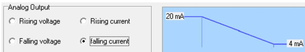
The analog output can be adjusted so that it supplies current or voltage. The characteristic can be selected as rising or falling.
