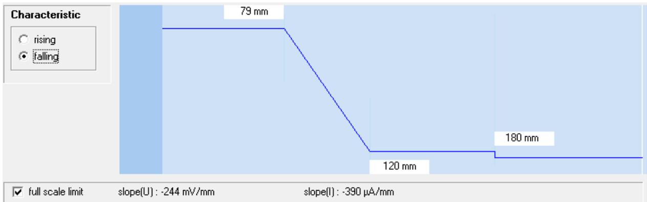
You can insert an additional break point behind the far sensor break point of the characteristic curve. Behind this break point the output voltage/output current falls to 0 V/4 mA.
