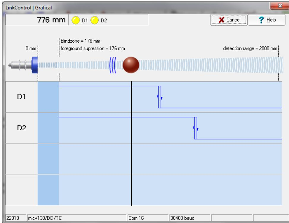
The displayed output characteristics correspond to the settings in the input mask.
