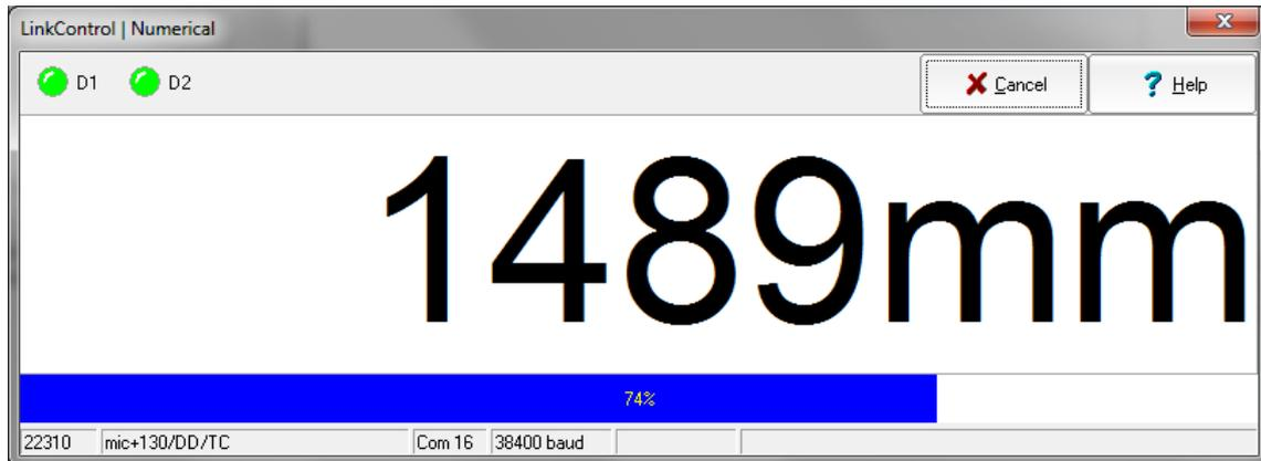
The measuring value is displayed in "mm" and as a bar graph in percent. The selected detection range is equivalent to 100%.
