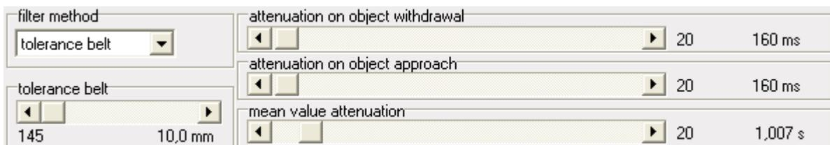
With this filter a tolerance belt is put symmetrically around the measured value. The current distance values remain within this belt, they are passed through an average filter.
