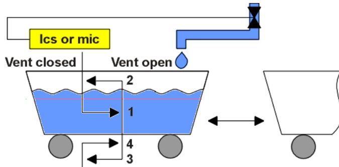
the output is set at trip distance 1 and the valve opens for filling. Beyond the hysteresis the valve closes again at trip distance 2. To prevent the valve from opening when there is no vehicle at all, the valve is kept shut by trip distance 3. As soon as there is a vehicle once again below the valve, the sensor re-opens the valve by trip distance 4.
