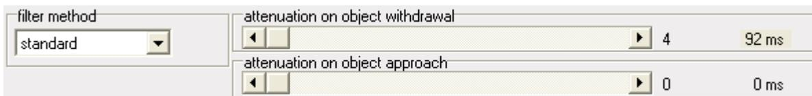
A screenshot of a software interface for the 'STANDARD – FILTER' settings. It features a 'filter method' dropdown menu set to 'standard'. Below it are two sliders: 'attenuation on object withdrawal' set to 4 with a 92 ms hold time, and 'attenuation on object approach' set to 0 with a 0 ms hold time.
