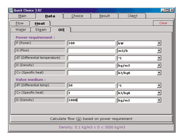
Click the **Calculate flow (G) based on power requirement** button at the bottom. Please see chapter 5 Calculations based on flow for further procedures.
