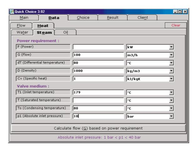
Click the **Calculate flow (G) based on power requirement** button at the bottom. Please see chapter 7 Calculations based on steam flow for further procedures.
