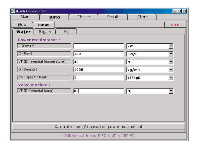
Click the **Calculate flow (G) based on power requirement** button at the bottom. Please see chapter 5 Calculations based on flow for further procedures.
