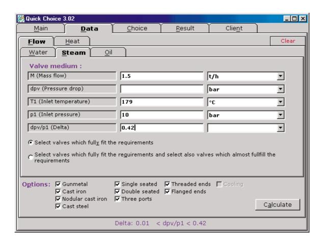
If necessary, deselect valve types or materials that are not desired, by clicking on the X 'es in the **Option** box.
