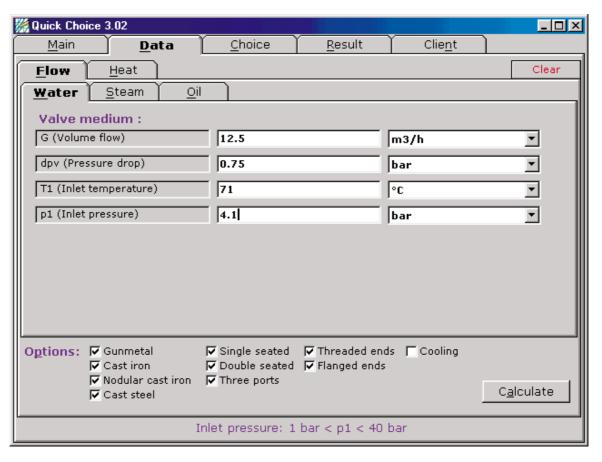
If units are to be changed, click the down-arrow button to the right of the Valve medium boxes. If necessary, deselect valve types or materials that are not desired, by clicking on the X'es under **Option**.
