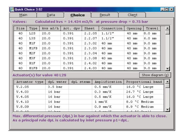
Now two lists appear. The top list contains valves which are close to the design requirements. The bottom list contains possible thermostats, motors and pressure differential controllers which may be connected to the valve to which the cursor points in the top list.
