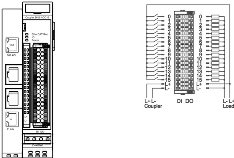
Front view of BK DI16/DO16 1MS/0.5A I/O module I/O connection
