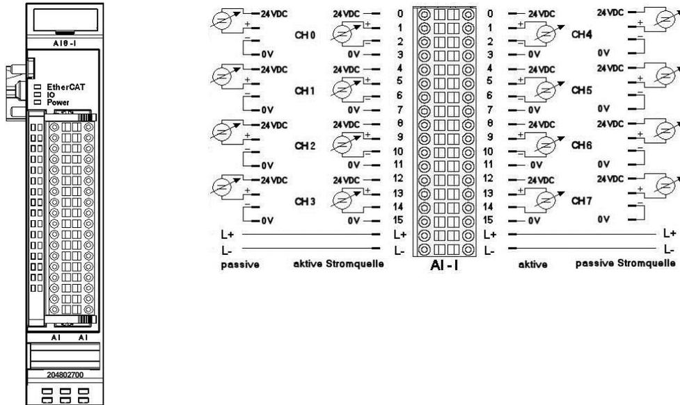
Front view of AI8-I I/O module I/O connection passive/active power source
