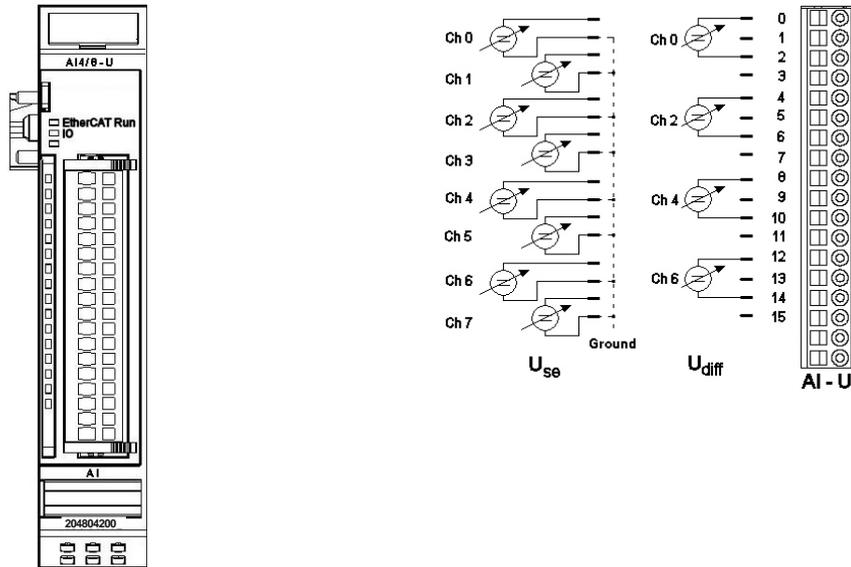
Front view of AI4/8-U 13BIT CoE I/O module I/O connection
