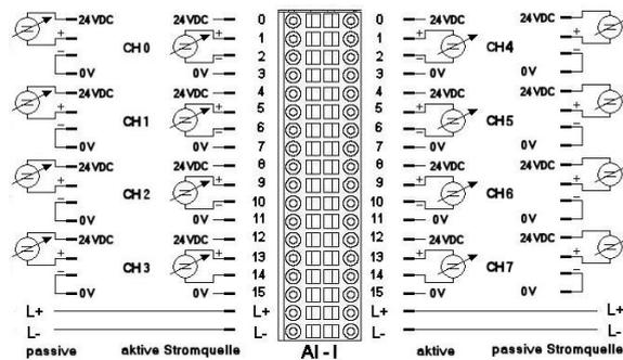
Front view of AI8-I 12BIT CoE I/O module      I/O connection
