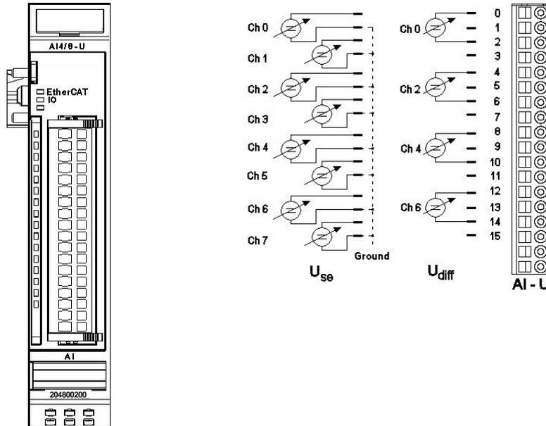
Front view of AI4/8-U I/O module    I/O connection
