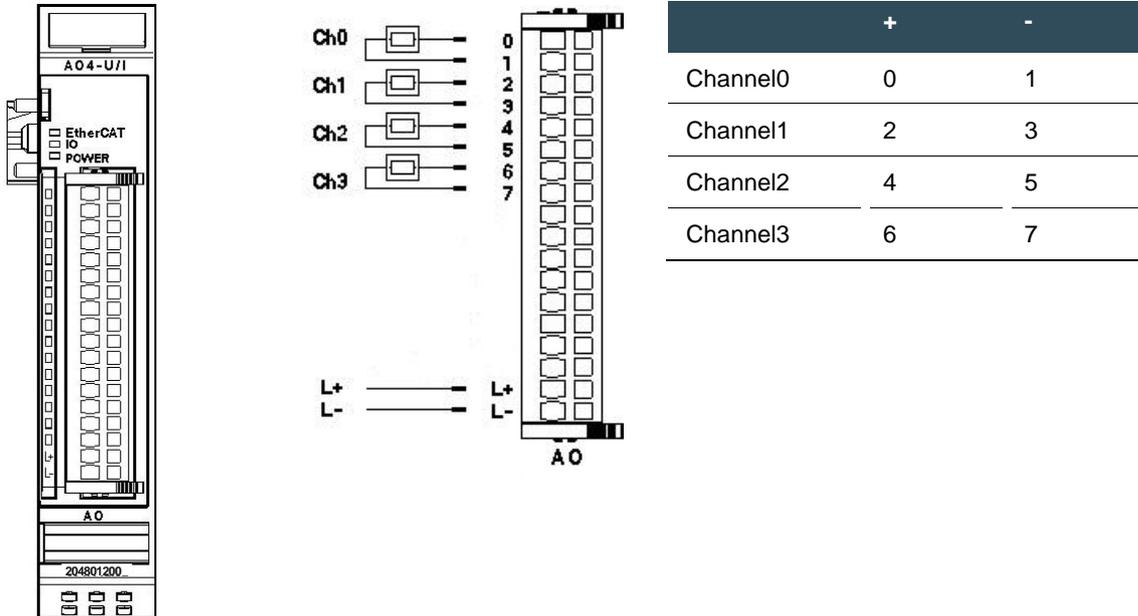
Front view of AO4-U/I I/O module    I/O connection
