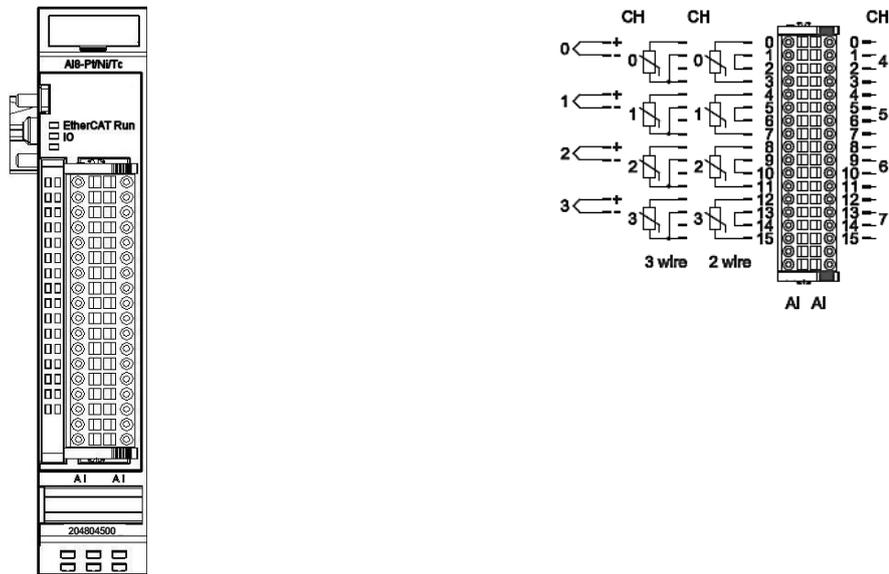
Front view of AI8-PT/NI/THERMO 16BIT CoE I/O module I/O connection
