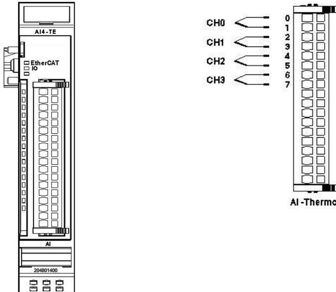
Front view of AI4-THERMO I/O module      I/O connection
