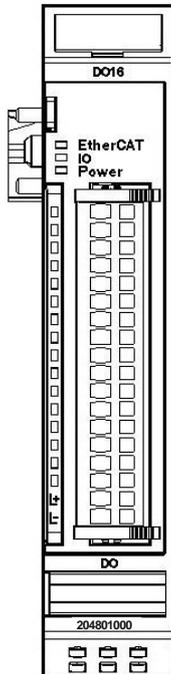
Front view of DO16 I/O module
