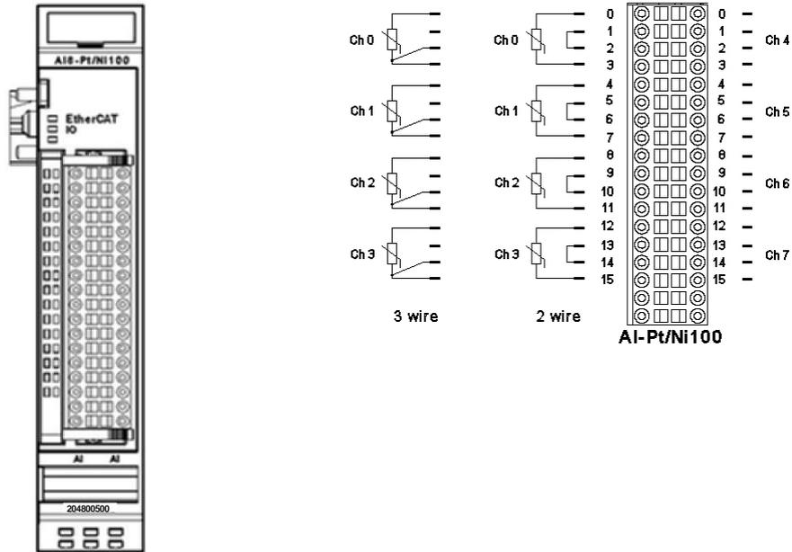
Front view of AI8-PT/Ni100 I/O module I/O connection
