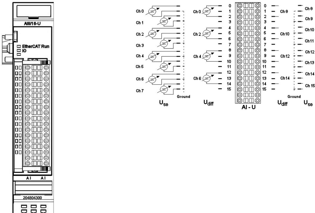
Front view of AI8/16-U 13BIT CoE I/O module I/O connection
