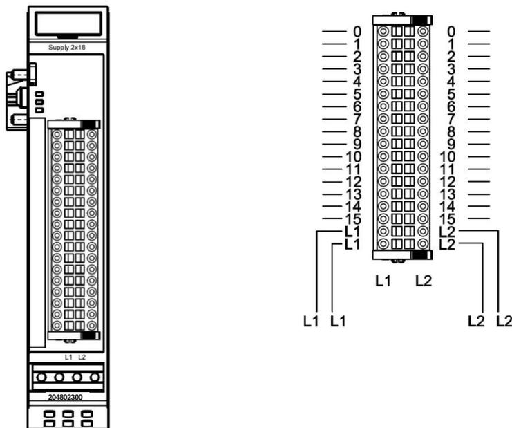
Front view of POTENTIALVERTEILER 2x16      Connections
