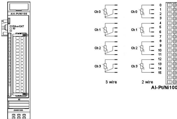
Front view of AI4-PT/Ni100 I/O module I/O connection
