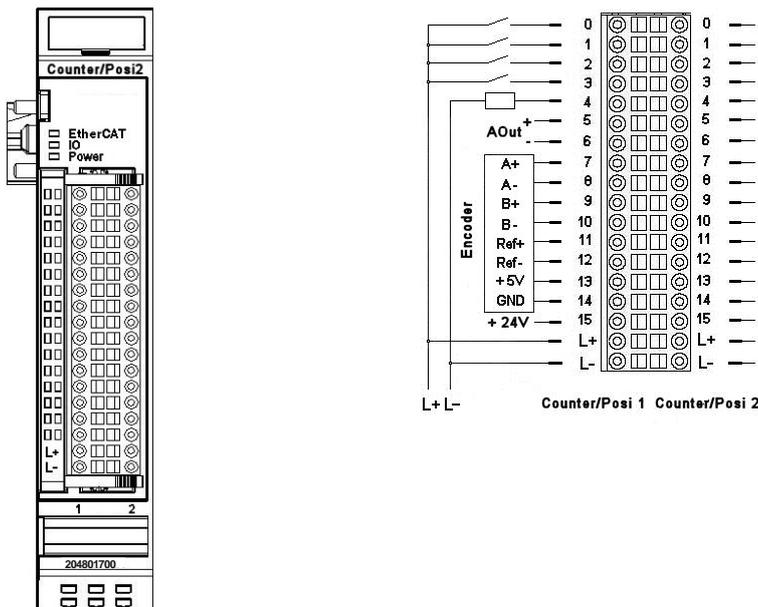
Front view of COUNTER/POSI2 5V I/O module    Pinning COUNTER/POSI2
