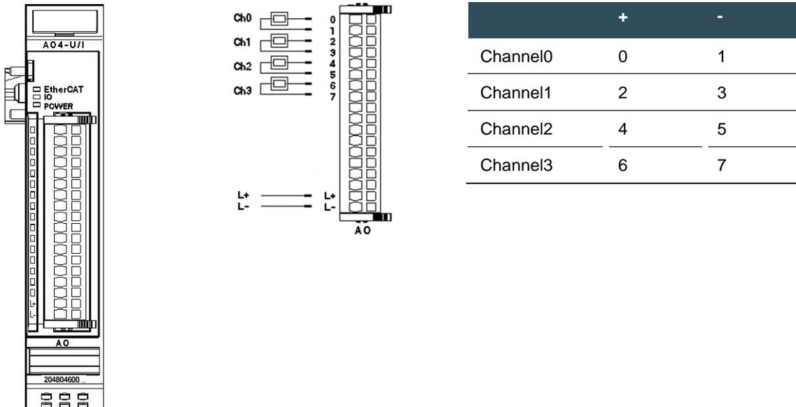
Front view of AO4-U/I 16BIT CoE I/O module
