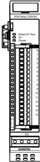
Front view of DO8 RELAIS NO 230VAC I/O module
