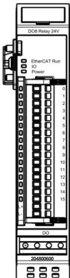
Front view of DO8 RELAIS NO 24V I/O module
