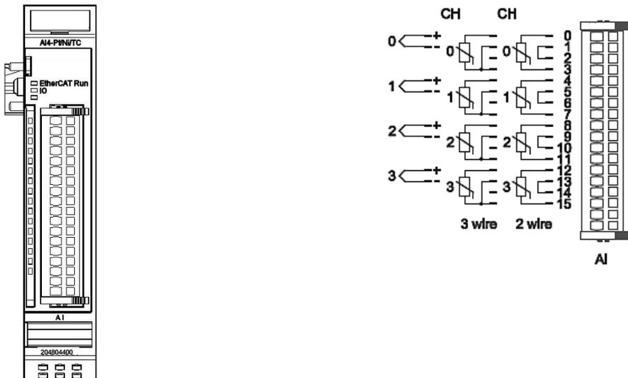
Front view of AI4-PT/NI/THERMO 16BIT CoE I/O module I/O connection
