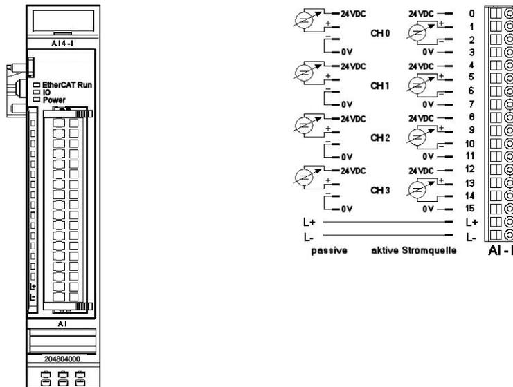
Front view of AI4-I 12BIT CoE I/O module    I/O connection
