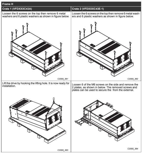
Tab. 2-10: Unpacking inverters of frame size H
