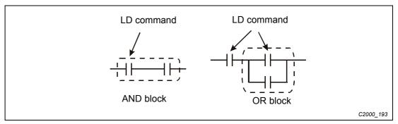
Fig. 16-23: LD command; the LDI command uses a normally closed contact
