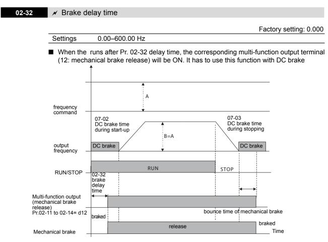
If this parameter is used without DC brake, it will be invalid. Refer to the following operation timing.
