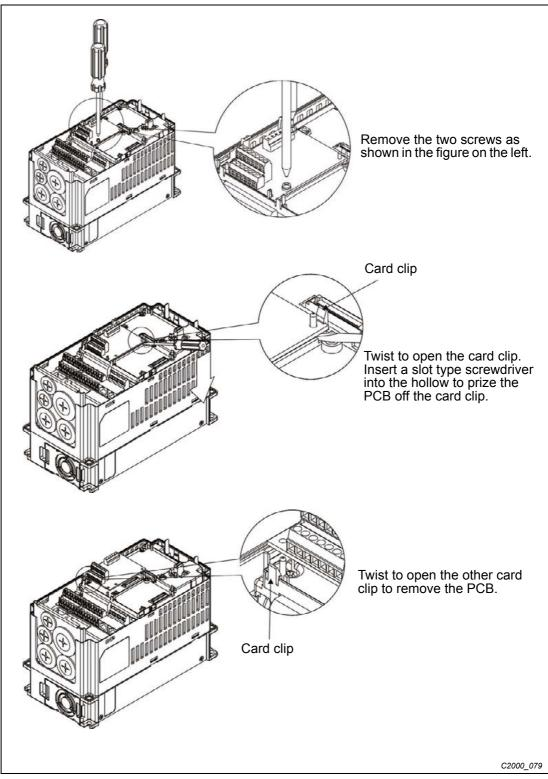
Fig. 8-15: Disconneting the extension card
