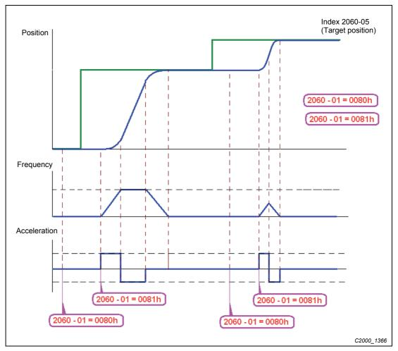
Fig. 15-11: Example for position control by the new Delta standard
