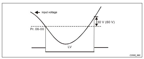
Fig. 12-39: Trigger threshold for low voltage
