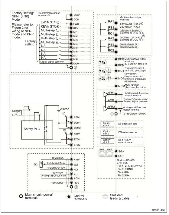
Fig. 4-3: Wiring of the input/output terminals
