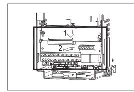
Fig. 6-4: Removing the control board
