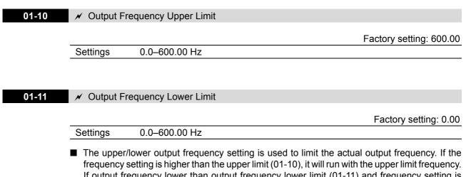
If output frequency lower than output frequency lower limit (01-11) and frequency setting is higher than min. frequency (01-07), it will run with lower limit frequency. The upper limit frequency should be set to be higher than the lower limit frequency. Pr. 01-10 setting must be  $\geq$  Pr. 01-11 setting.
