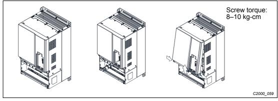
Fig. 8-2: Cover removal and screw tightening torque
