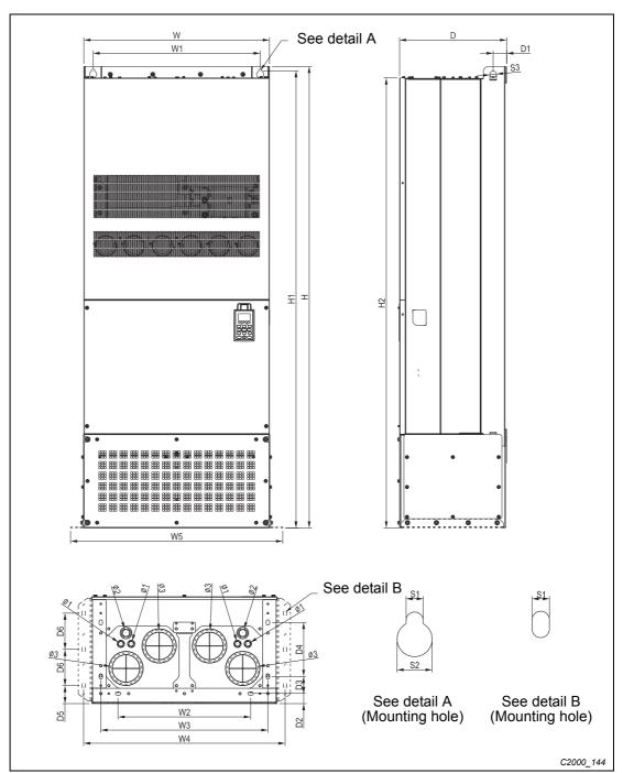
H3: VFD2800C43E, VFD3150C43E, VFD3550C43E
