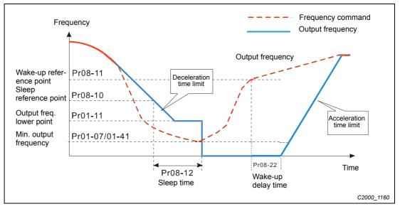
Fig. 12-69: Internal PID calculation frequency command
