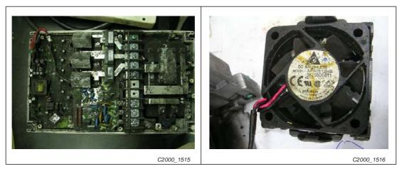
Fig. 18-1: Greasy dirt inside the frequency inverter and at the cooling fans
