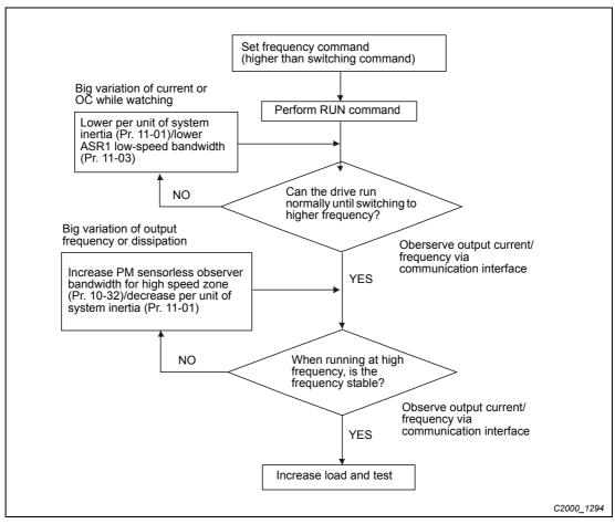
Fig. 12-75: Procedure for switching between I/F mode and FOC mode
