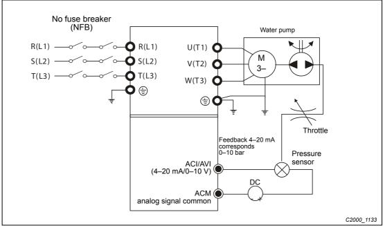
Fig. 12-65: Constant pump pressure control
