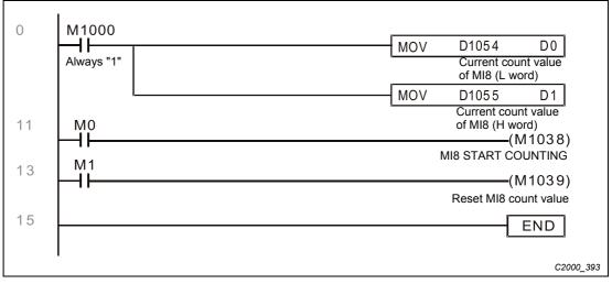
Fig. 16-40: Program example for high-speed count function using MI8
