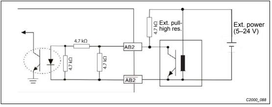
Fig. 8-23: Wiring diagram of open collector encoder with external power supply
