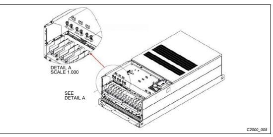
Fig. 5-5: Short circuit plate removement
