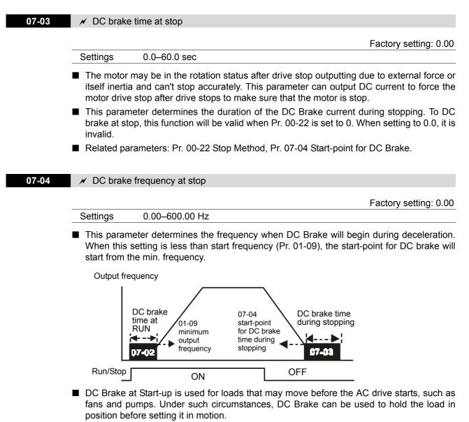
■ DC Brake at stop is used to shorten the stopping time and also to hold a stopped load in position, such as crane or cutting machine.
