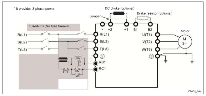
Fig. 4-1: Inverter wiring diagram for frame size A-C
