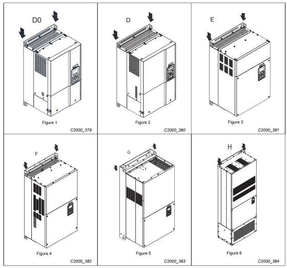
Tab. 2-18: Lifting the inverter
