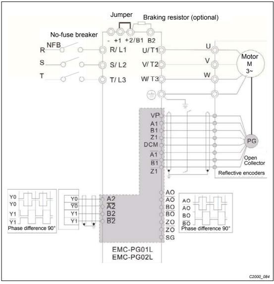
Fig.8-19: Wiring diagram of option card EMC-PG01L/EMC-PG02L
