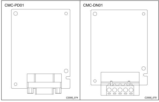
Fig. 8-12: Communication extension card (Slot 1)
