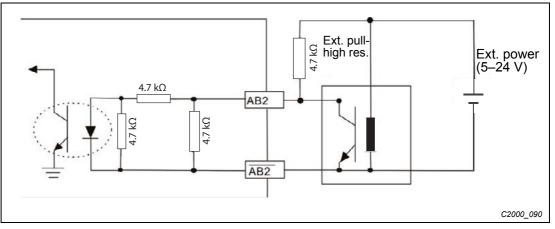
Fig.8-25: Wiring diagram of open collector encoder with external power supply
