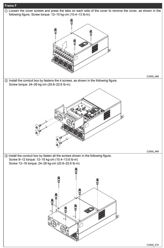
Tab. 7-27: Installation of the conduit box to frame F
