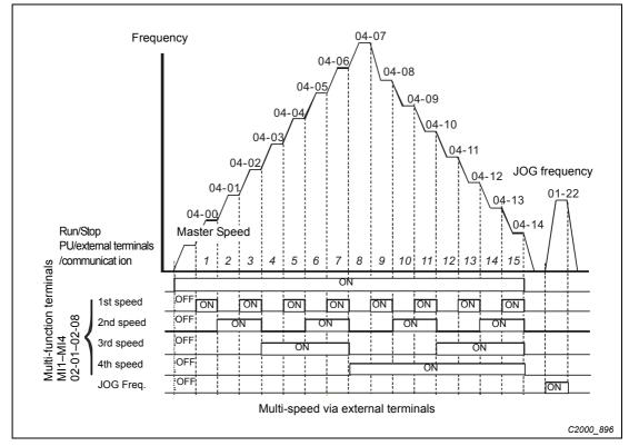
Fig. 12-34: Speed selection via external terminals
