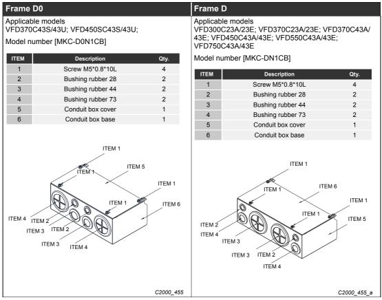
Tab. 7-21: Conduit box for frames D0 and D
