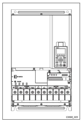
Fig. 5-17: View of frequency inverter frame D
