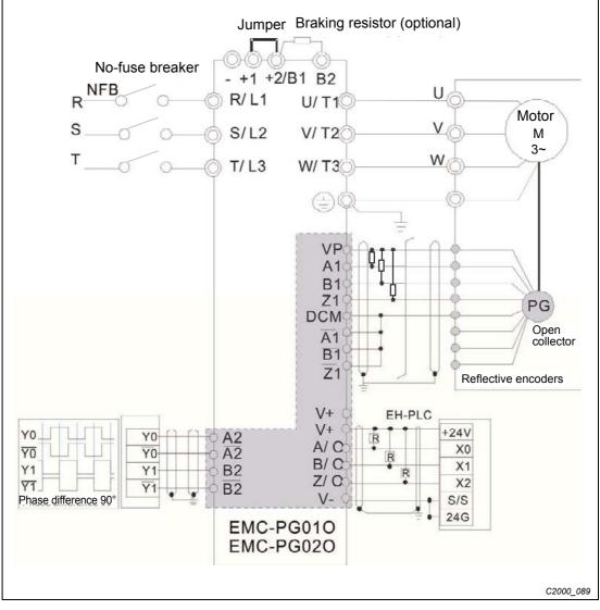
Fig. 8-24: Wiring diagram of option card EMC-PG01O/EMC-PG02O
