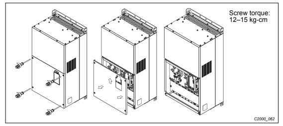
Fig. 8-5: Cover removal and screw tightening torque
