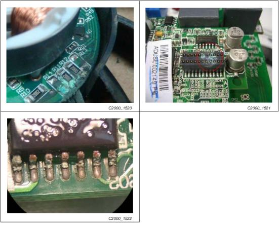
Fig. 18-3: Damage from corrosion
