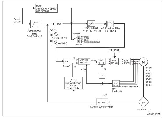
Fig. 12-5: IM FOCPG control diagram
