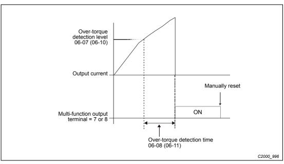
Fig. 12-44: Operation stop at over-torque
