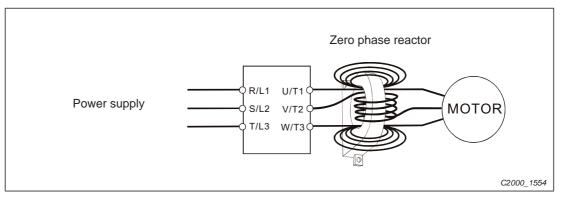
Fig. 19-20: The motor wire is winded through the middle of the zero phase reactor
