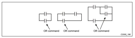
Fig. 16-26: OR command; the ORI command uses a normally closed contact
