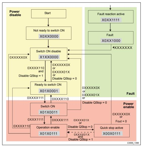
Fig. 15-4: Fault processing and status messages
