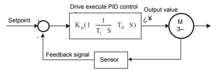
K<sub>p</sub>: Proportional gain (P) T<sub>i</sub>: Integral time (I) T<sub>d</sub>: Derivative control (D) S: Operator
