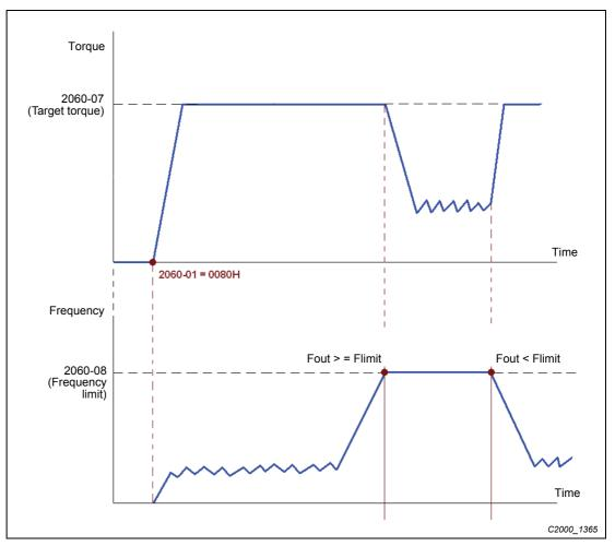
Fig. 15-10: Example for torque control by the new Delta standard
