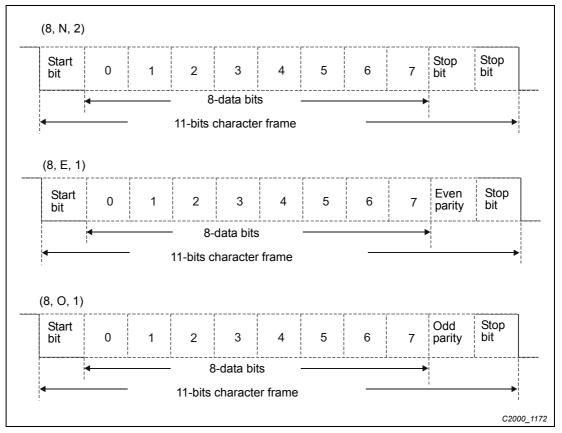
Fig. 12-72: 11-bit character frame (for RTU)
