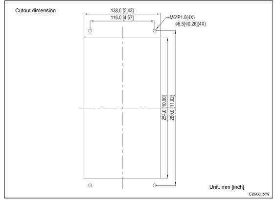
Fig. 7-15: Cutout dimension for plate installation
