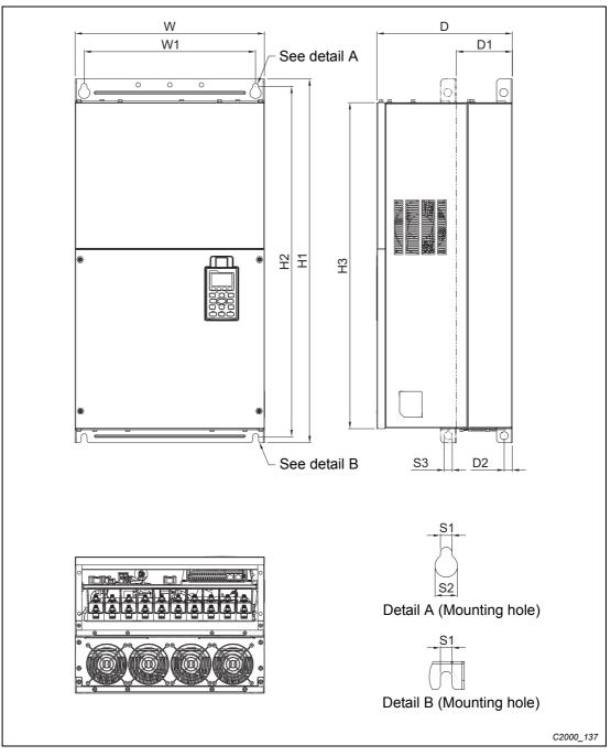
F1: VFD900C23A, VFD1320C43A, VFD1600C43A
