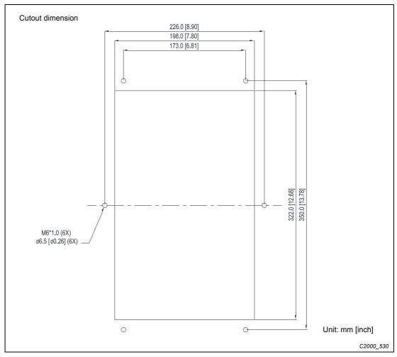
Fig. 7-16: Cutout dimension for plate installation
