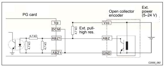
Fig. 8-17: Wiring diagram of open collector encoder with external power supply
