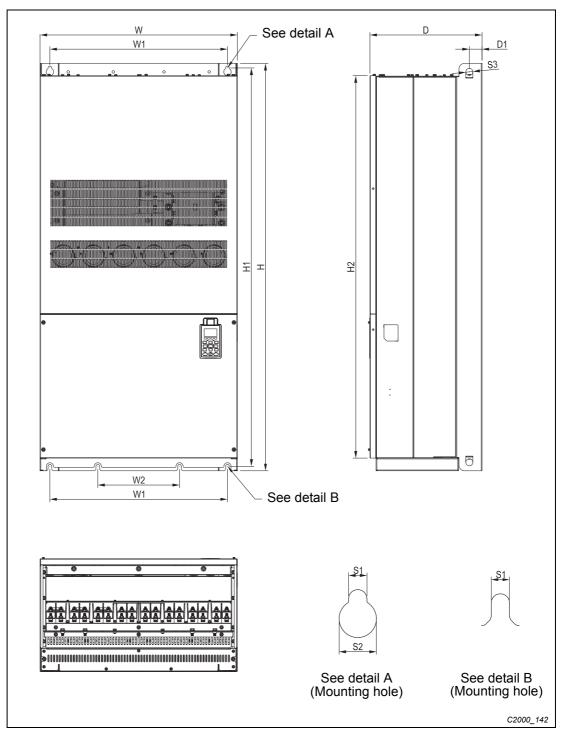
Fig. 1-26: Dimensions frame size H1
