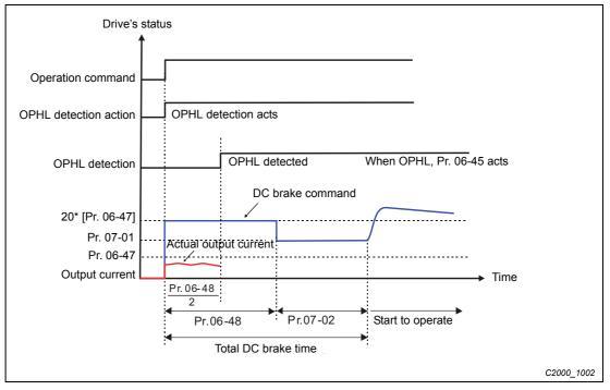
Fig. 12-50: Status 3-2: Pr. 06-48  $\neq$  0, Pr. 07-02  $\neq$  0 (OPHL detected before operation)
