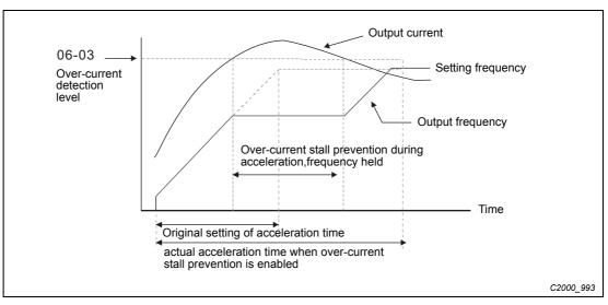
Fig. 12-41: Stall prevention at over-current during acceleration
