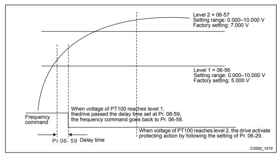
Fig. 12-63: Trigger threshold of PT100 sensor
