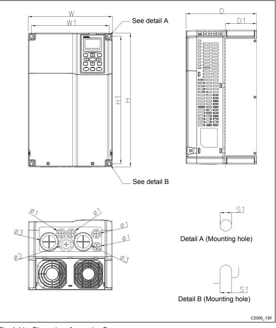
Fig. 1-14: Dimensions frame size C
