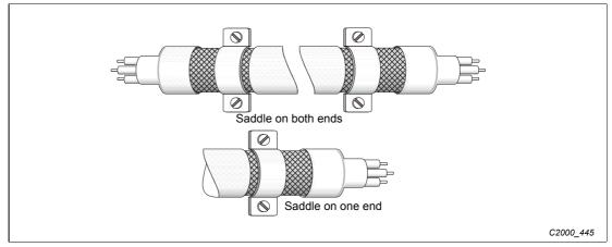
Fig. 7-6: Mounting of the saddles
