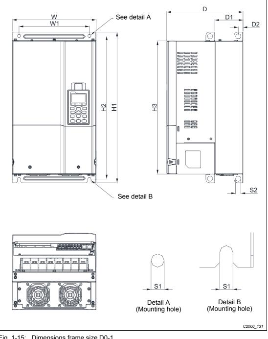
Fig. 1-15: Dimensions frame size D0-1
