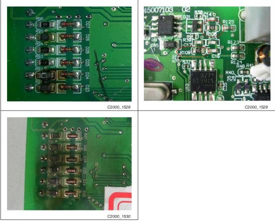
Fig. 18-6: Damage due to overload of the input/output terminals
