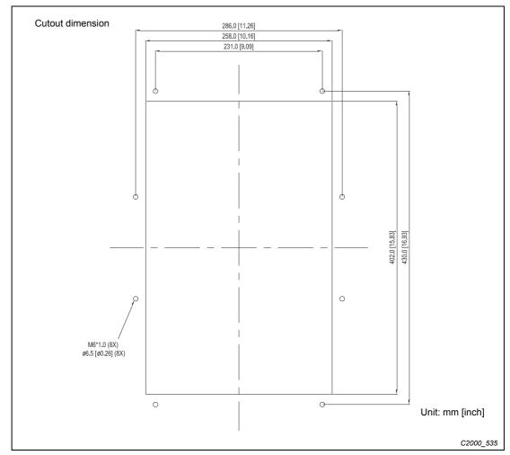
Fig. 7-17: Cutout dimension for plate installation
