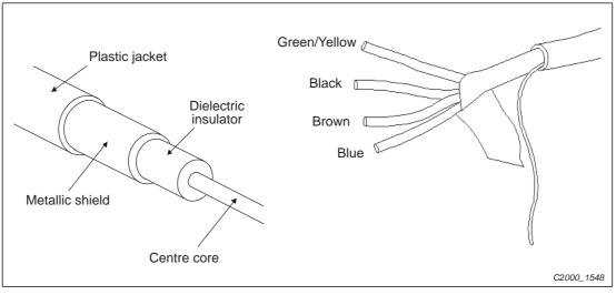
Fig. 19-16: Shielded cable structures
