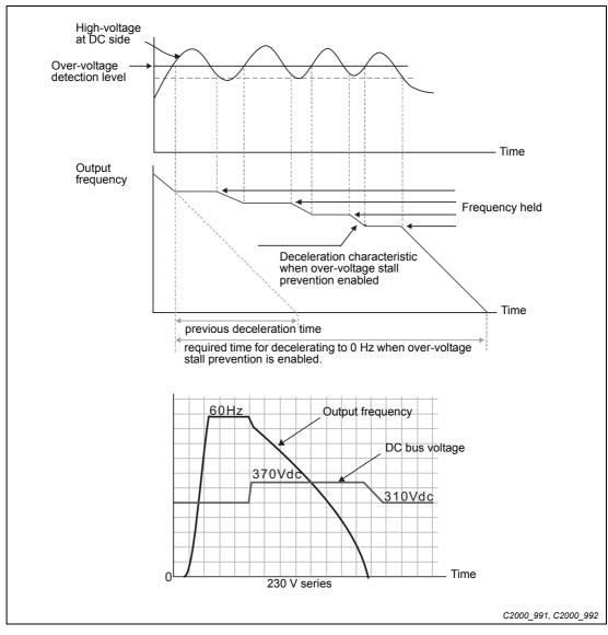
Fig. 12-40: Stall prevention at over-voltage
