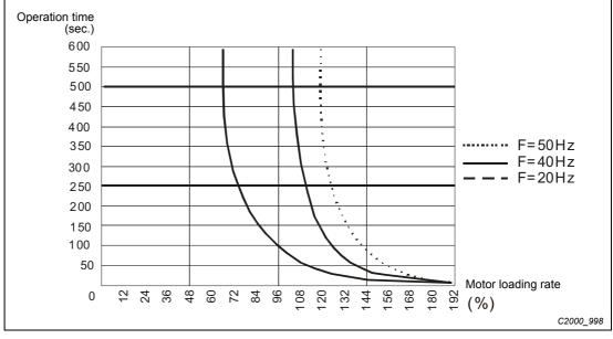
Fig. 12-46: Motor protection characteristics
