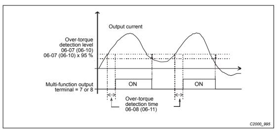
Fig. 12-43: Continuous operation at over-torque
