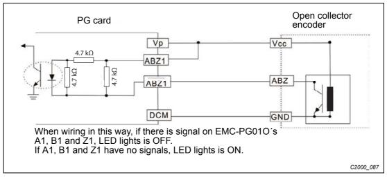
Fig. 8-22: Wiring diagram of open collector encoder
