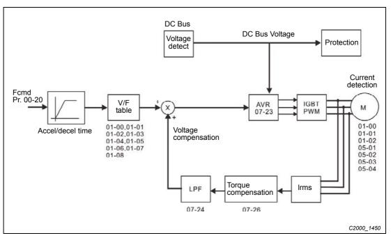
Fig. 12-2: V/F control diagramm
