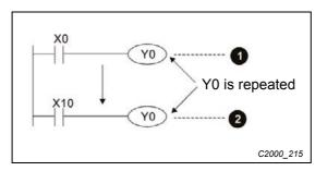
Fig.16-30: The output of Y0 will be decided by circuit (2), i.e. decided by On/ Off of X10.
