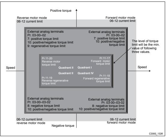
Fig. 12-78: Torque limiting in forward and reverse mode
