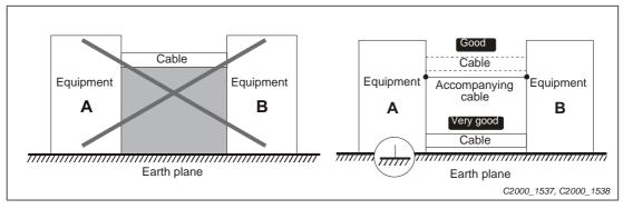
Fig. 19-7: EMC conform connection of two devices
