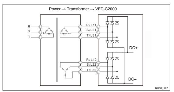
Fig. 5-4: Main circuit wiring diagram for frame G and above
