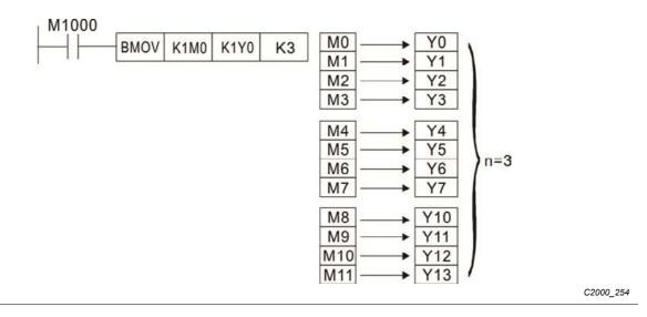
**EXAMPLE 3** In order to prevent overlap between the transmission addresses of two operands, which would cause confusion, make sure that the addresses designated by the two operands have different sizes, as shown below:
