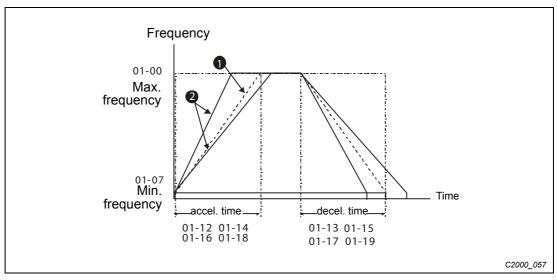
Fig. 12-26: Acceleration/deceleration time
