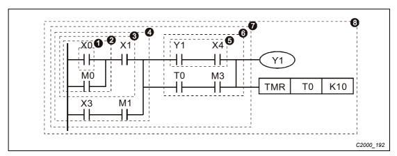
Fig. 16-22: Explanation of command sequence
