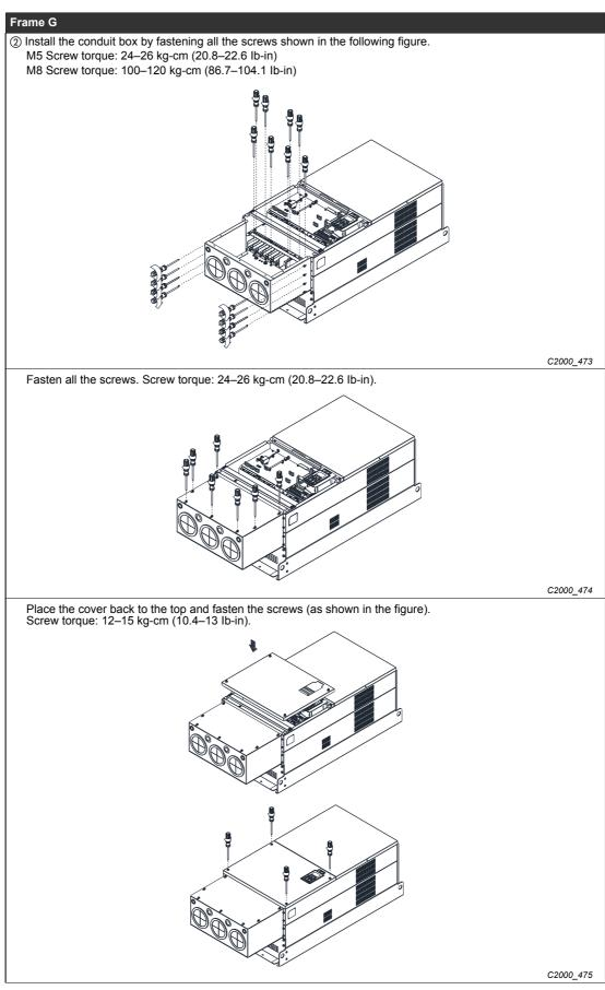
Tab. 7-29: Installation of the conduit box to frame G
