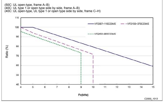
Fig. 12-61: Derating curve for sensorless control (230 V, HD)
