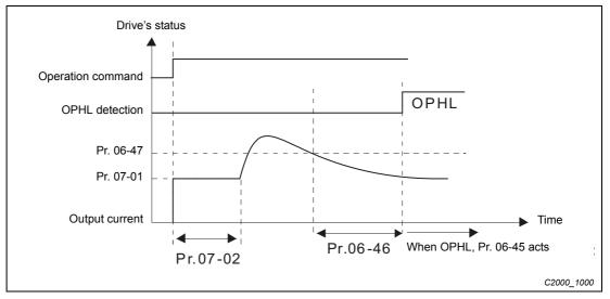
Fig. 12-48: Output phase loss (OPHL) during frequency inverter stop
