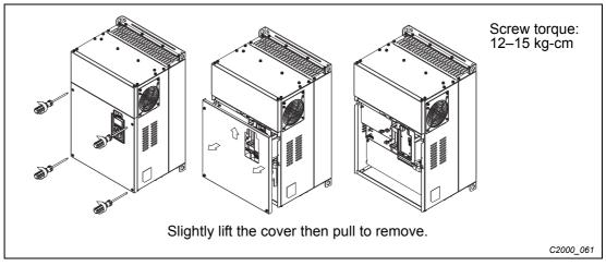
Fig. 8-4: Cover removal and screw tightening torque
