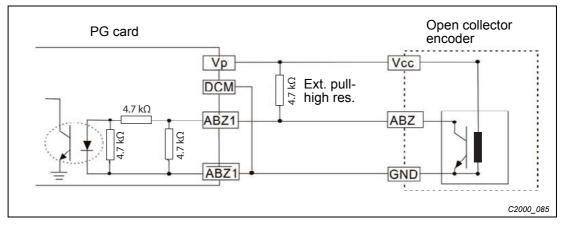
Fig. 8-20: Wiring diagram of open collector encoder
