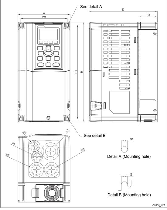
Fig. 1-12: Dimensions frame size A
