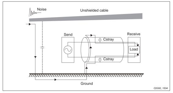
Fig. 19-4: Noise transmission to wire shields via stray capacitances
