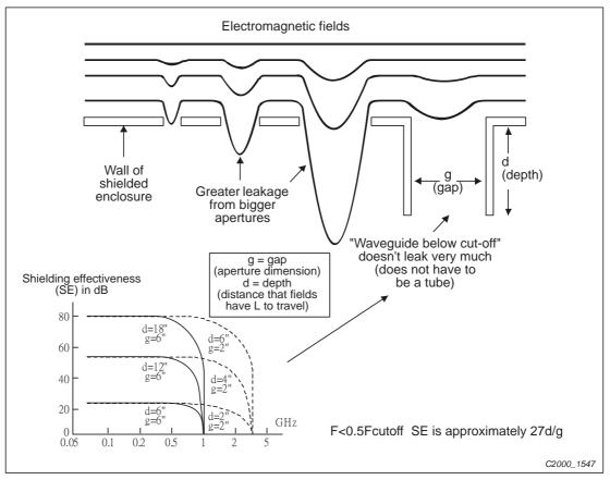
Fig. 19-15: Influence of the size of the holes and the depth to the shielding
