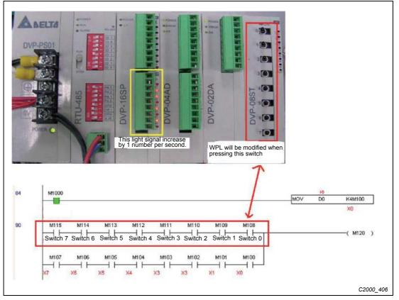
Fig. 16-47: Displaying the status of inputs and switches in WPLSoft
