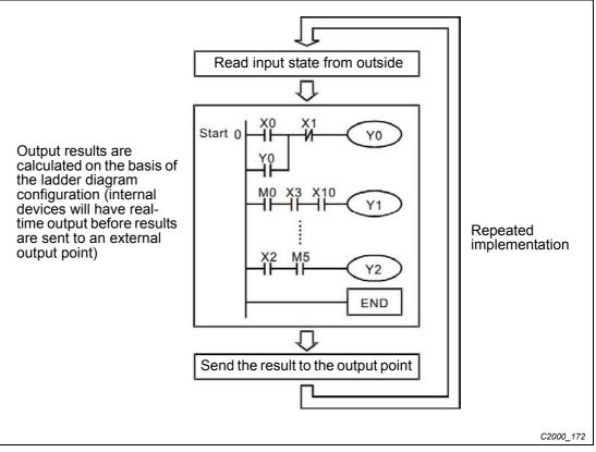
Fig. 16-20: Principle of cyclic program execution
