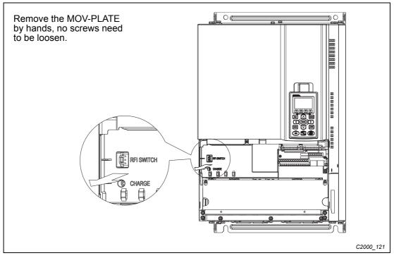
Fig. 1-5: Removal of the RFI jumper (frame size D-H)
