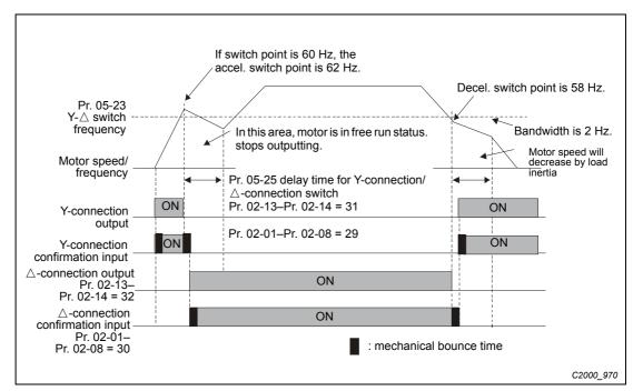
Fig. 12-37: Output signals at star/delta connection
