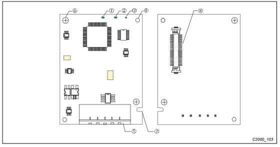
Fig. 8-37: View of the option card CMC-DN01
