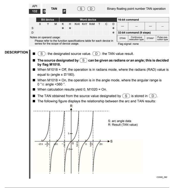
**EXAMPLE** When X0 = On, the TAN value of the designated binary floating point number (D1, D0) in radians (RAD) will be stored in (D11, D10), with the content consisting of a binary floating point number.
