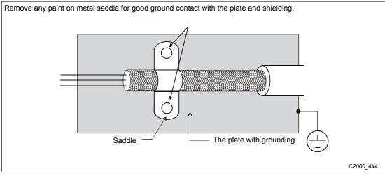
Fig. 7-5: Grounding of a shielded cable
