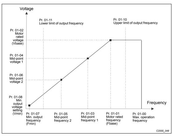
Fig. 12-18:Limit value ratio for output frequency
