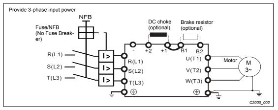
Fig. 5-2: Main circuit wiring diagram for frame A-C with DC choke
