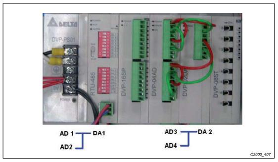
Fig. 16-48: For testing, the analog inputs and outputs are connected.
