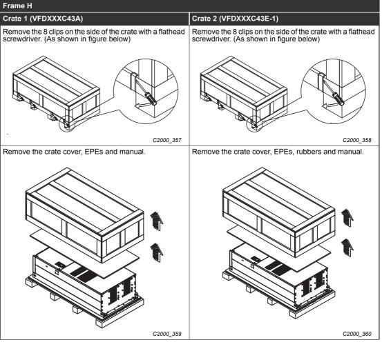
Tab. 2-9: Unpacking inverters of frame size H
