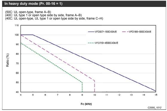
Fig. 12-60: Derating curve for sensorless control (460 V, HD)
