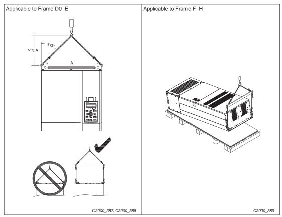
Fig. 2-2: Correct lifting method
