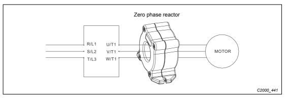
Fig. 7-4: Wiring of the zero phase reactor
