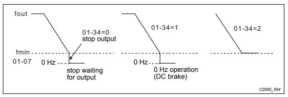
Fig. 12-23:Zero-speed process
