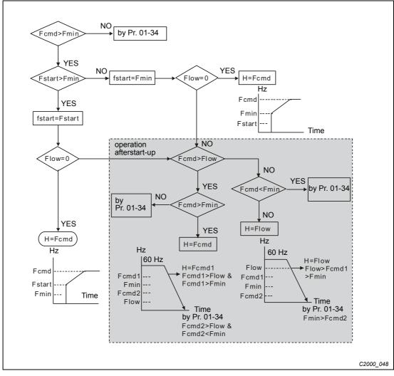
Fig. 12-17: Start-up frequency flowchart
