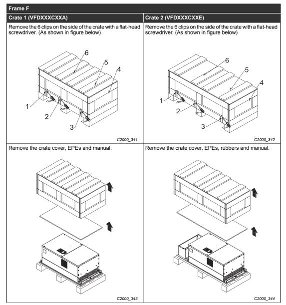
Tab. 2-5: Unpacking inverters of frame size F
