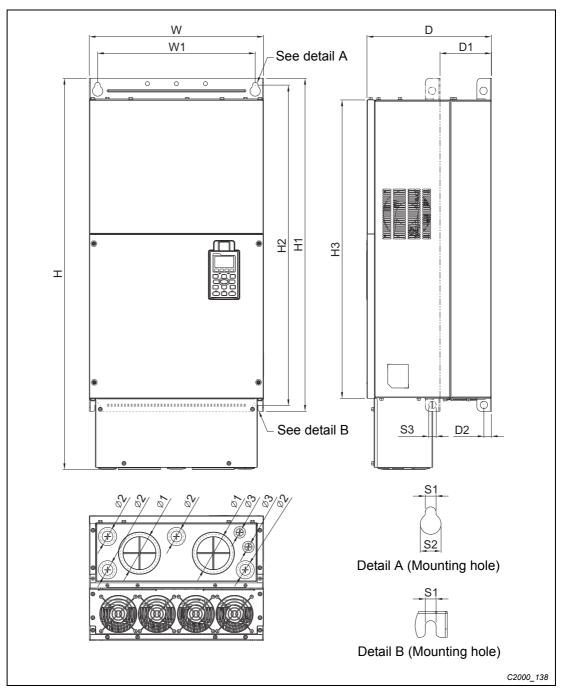
F2: VFD900C23E, VFD1320C43E, VFD1600C43E
