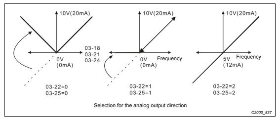
Fig. 12-33: Selection of the revolution direction for the analog inputs
