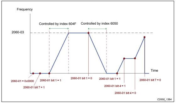
Fig. 15-9: Example for speed control by the new Delta standard
