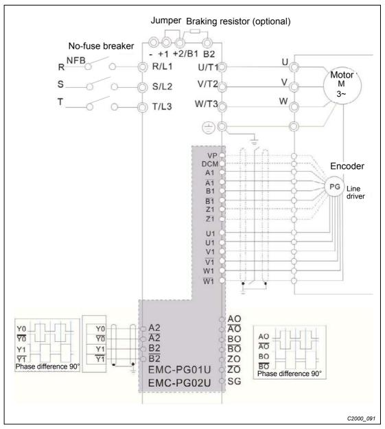
Fig.8-26: Wiring diagram of option card EMC-PG01U
