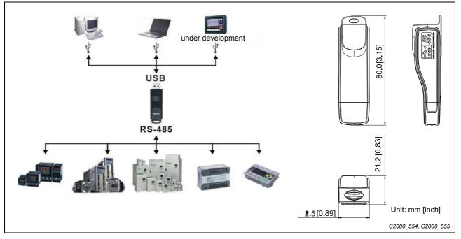
Fig. 7-18: Interface converter IFD6530
