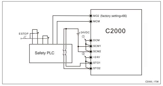
Fig. 20-3: Security circuit with safety PLC
