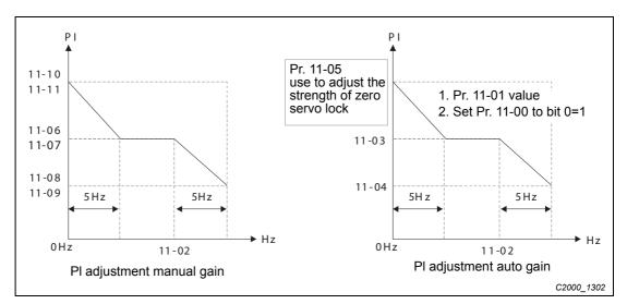
Fig. 12-77: PI gain adjustment
