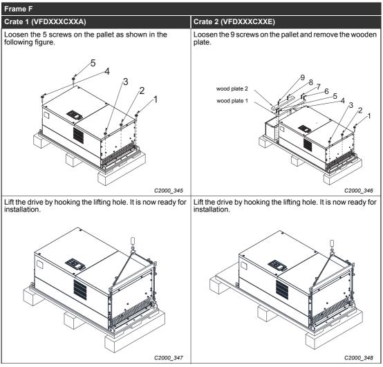
Tab. 2-6: Unpacking inverters of frame size F
