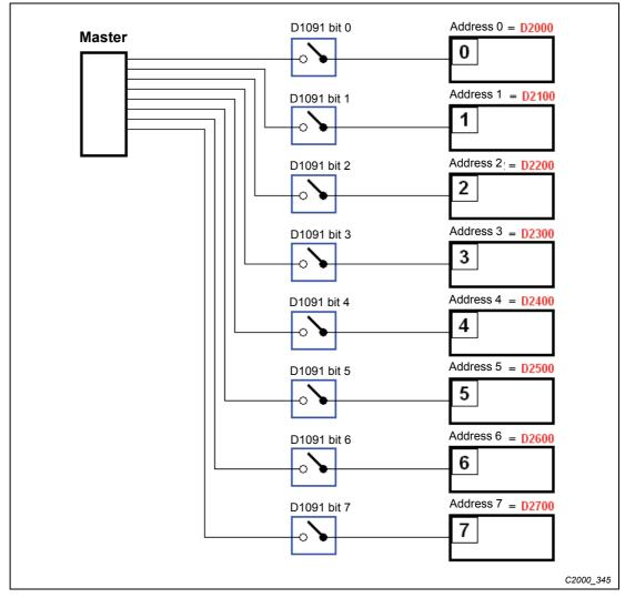
Fig. 16-36: The contents of D1091 determines the slave to communicate with
