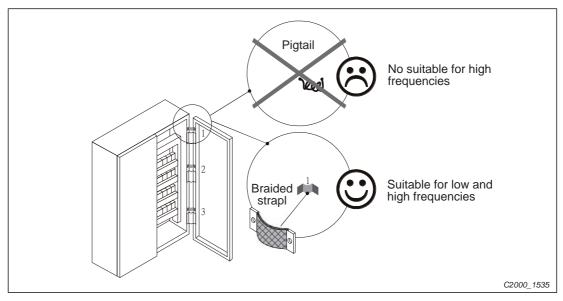
Fig. 19-5: Door connection of a control cabinet with a ground strap.
