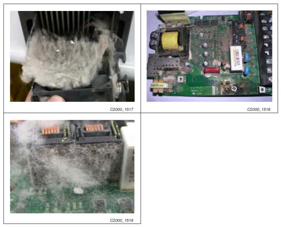
Fig. 18-2: Collection of fiber dust inside the frequency inverter
