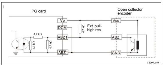
Fig. 8-16: Wiring diagram of open collector encoder
