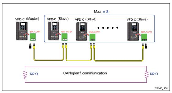
Fig. 16-38: Example for the connection of VFDs via CAN
