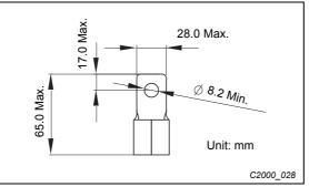
Fig. 5-22: Ring lug grounding wire
