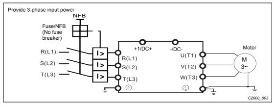
Fig. 5-3: Main circuit wiring diagram for frame D0 and above
