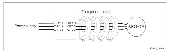
② Place all wires through the middle of four zero-phase reactors without winding.
