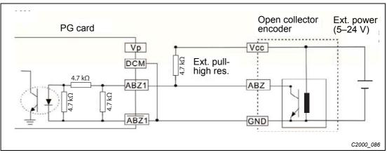
Fig. 8-21: Wiring diagram of open collector encoder with external power supply
