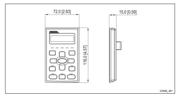
Fig. 7-8: Dimensions of the digital keypad
