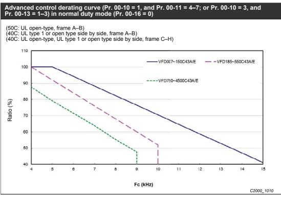
Fig. 12-58: Derating cureve for sensorless control (460 V, ND)
