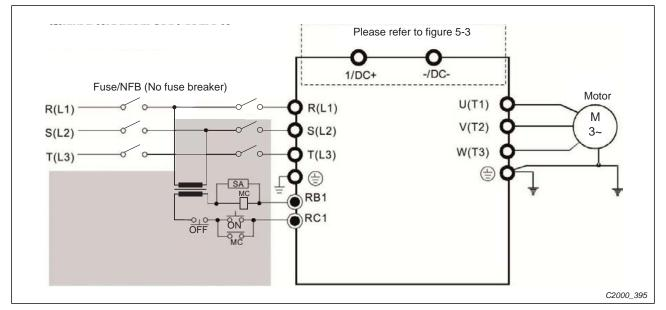
Fig. 4-2: Inverter wiring diagram for frame size D and above
