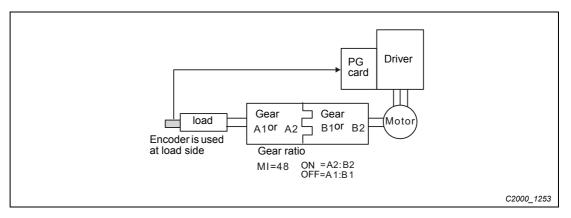
Fig. 12-73: Gear with encoder at the load side
