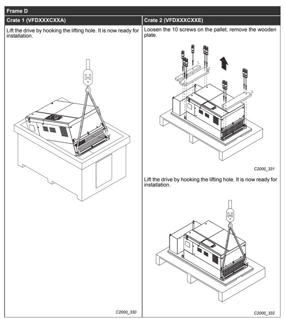
Tab. 2-2: Unpacking inverters of frame size D
