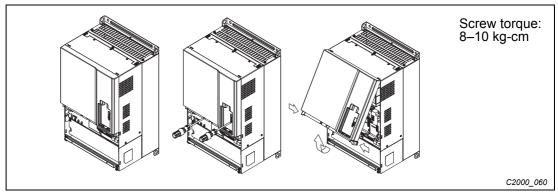
Fig. 8-3: Cover removal and screw tightening torque
