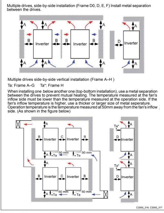
Fig. 3-2: Minimum mounting clearances
