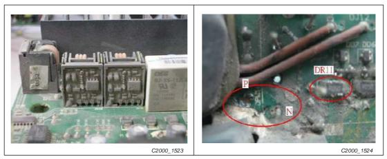
Fig. 18-4: Residue of industrial dust inside the frequency inverter
