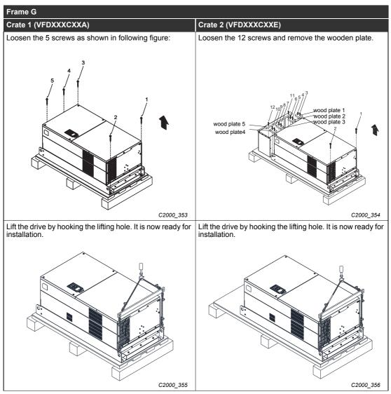
Tab. 2-8: Unpacking inverters of frame size G
