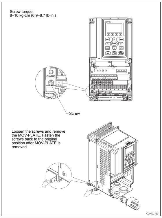
Fig. 1-4: Removal of the RFI jumper (frame size A-C)
