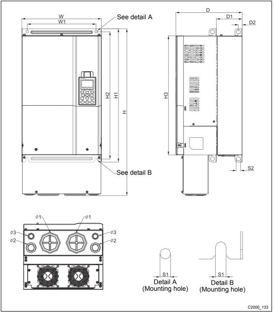
D1: VFD300C23A, VFD370C23A, VFD550C43A, VFD750C43A
