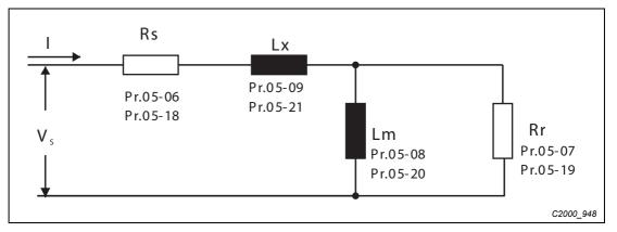
Fig. 12-35: Motor replacement circuit diagram
