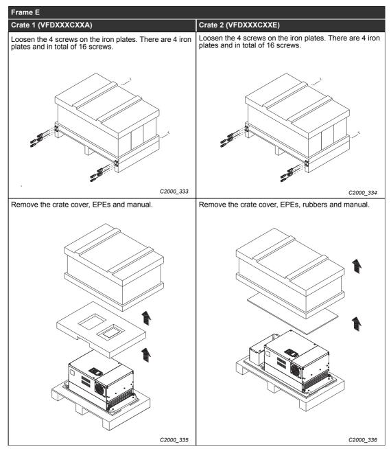
Tab. 2-3: Unpacking inverters of frame size E
