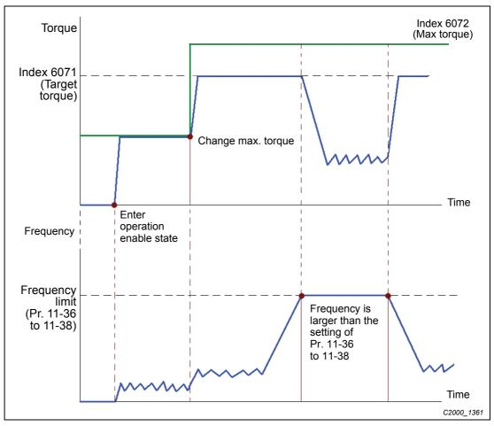
Fig. 15-6: Example for torque control
