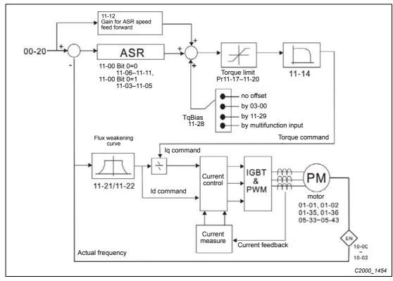
■ When 00-10 = 0, and set Pr. 00-11 to 4, the PM FOCPG control diagram is shown as follows:
