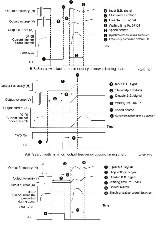
B.B. Search with minimum output frequency upward timing chart C2000\_1103
