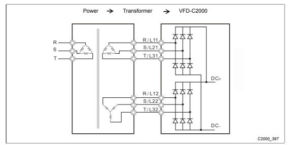
Fig. 4-4: Main circuit wiring diagram for framesize G and above
