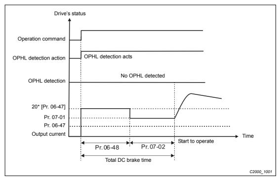
Fig. 12-49: Status 3-1: Pr. 06-48  $\neq$  0, Pr. 07-02  $\neq$  0 (No OPHL detected before operation)
