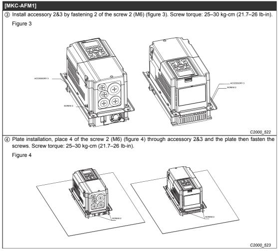
Tab. 7-34: Mounting of accessories and plate installation
