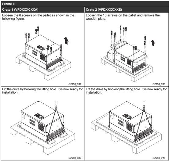
Tab. 2-4: Unpacking inverters of frame size E
