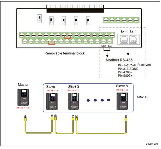
Fig. 16-39: Connection between master stations and slave stations
