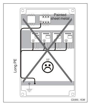
Fig.19-6: A long ground wire is bad at high frequencies
