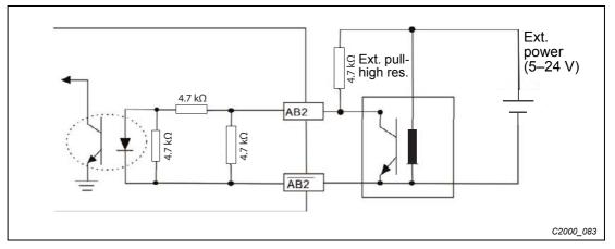
Fig. 8-18: Wiring daigram of open collector encoder
