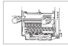
Fig. 6-3: Removing the screws
