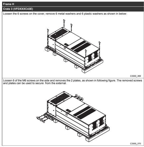
Tab. 2-13: Unpacking inverters of frame size H
