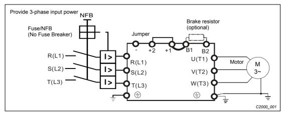
Fig. 5-1: Main circuit wiring diagram for frame A-C
