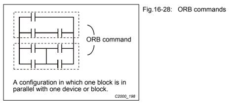
In the case of ANB and ORB operations, if a number of blocks are connected, they should be combined to form a block or network from the top down or from left to right.
