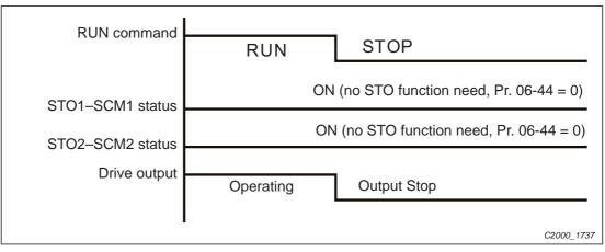
Fig. 20-4: Signal course at normal operation
