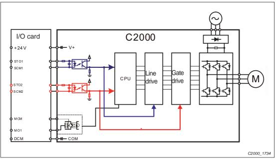
Fig. 20-1: Block diagram of the internal STO circuit
