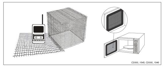
Fig. 19-14: Shielding of radio waves (left) and micro waves (right)
