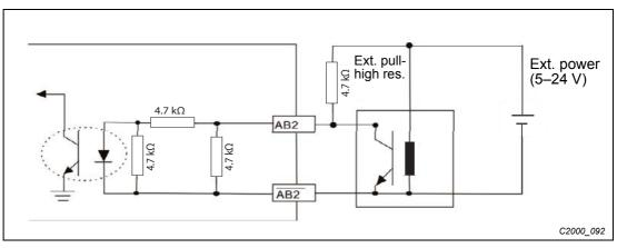
Fig.8-27: Wiring diagram of open collector encoder with external power supply
