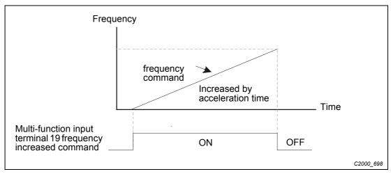
Fig. 12-28: Frequency set value at Pr. 02-09 = 1
