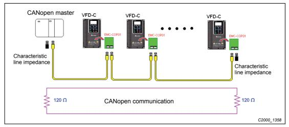
Fig. 15-3: Frequency inverter connection via CAN-Bus
