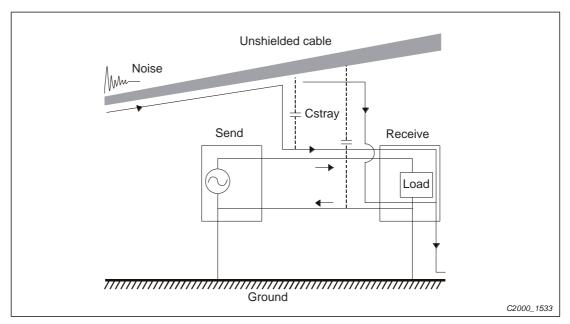
Fig. 19-3: Noise transmission to other systems via stray capacitances
