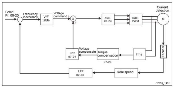
Fig. 12-3: V/F control and encoder diagram
