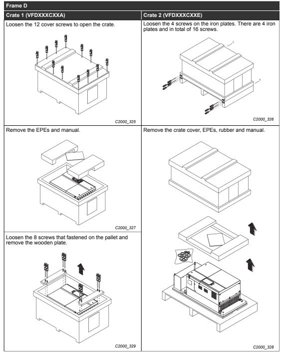
Tab. 2-1: Unpacking inverters of frame size D
