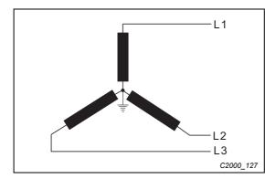
Fig. 1-11: Symmetrical grounding power system (star configuration)
