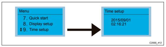
Fig. 16-50: Setting the time and date on the keypad KPC-CC01
