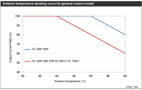
Fig. 12-57: Derating for high ambient temperature
