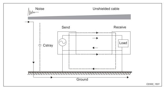
Fig. 19-1: Noise transmission to the ground via stray capacitances
