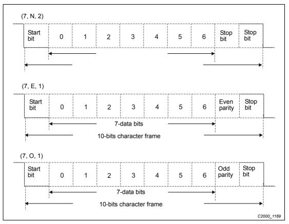
Fig. 12-71: 10-bit character frame (for ASCII)
