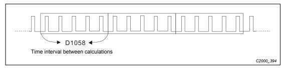
Fig. 16-41: Example for pulses on terminal MI8 of the variable frequency drive
