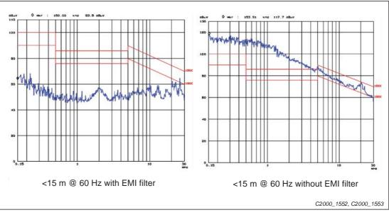
Fig. 19-19: Interferences (blue line) will be supressed by a noise filter
