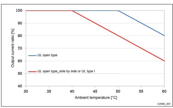
Normal control ambient temperature derating curve
