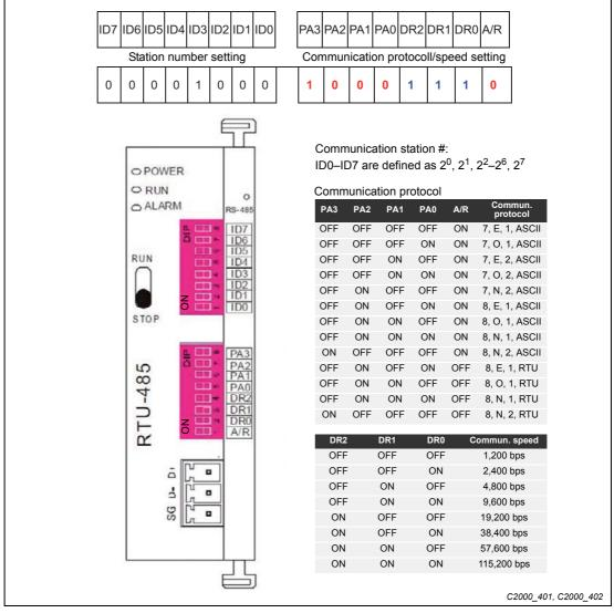
Fig. 16-43: Setting of station number, communication protocol, and communication speed
