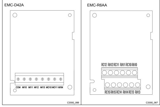
Fig. 8-8: I/O & relay extension card (Slot 3)
