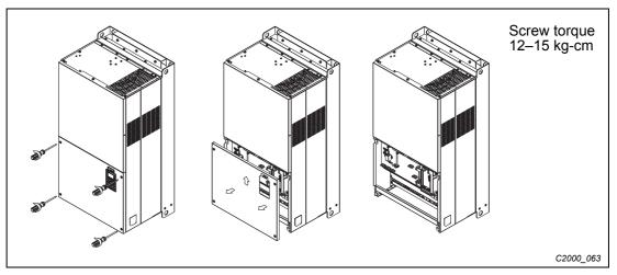
Fig. 8-6: Cover removal and screw tightening torque
