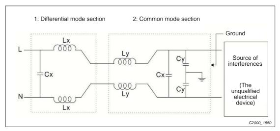
Fig. 19-17: Typical wire diagram of a noise filter
