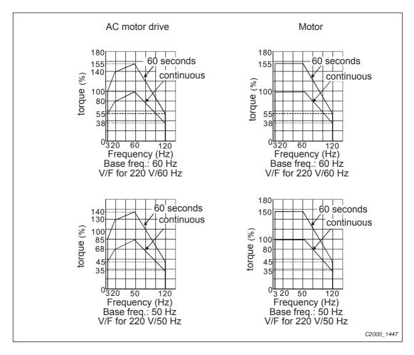
Fig. 17-2: Torque-speed characteristics of a standard motor (4-pole, 15 kW)
