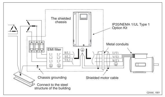
Fig. 19-18: Installation of an external noise filter
