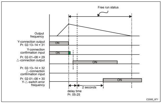
Fig. 12-38: Error at missing confirmation signal
