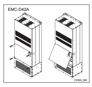
Fig. 8-7: Cover removal and screw tightening torque: 14–16 kg-cm
