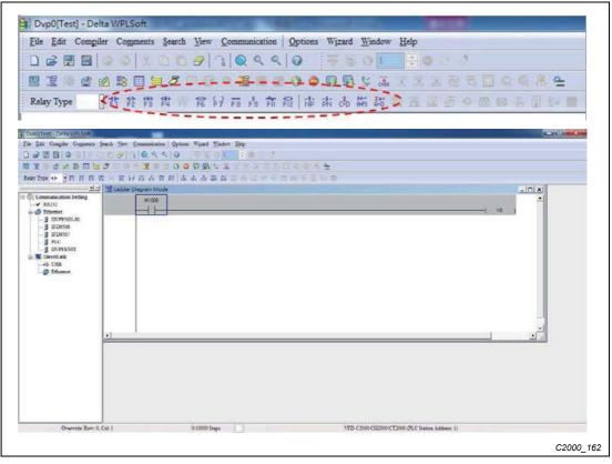
Fig. 16-12: Symbols for ladder programs in the tool bar
