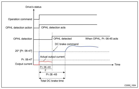
Fig. 12-52: Status 4-2: Pr. 06-48  $\neq$  0, Pr. 07-02 = 0 (OPHL detected before operation)
