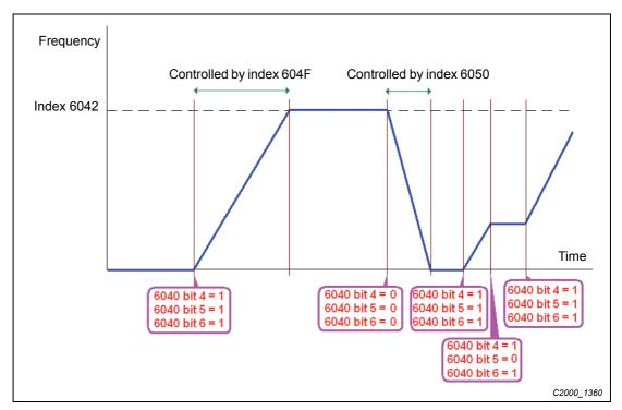
Fig. 15-5: Example for speed control
