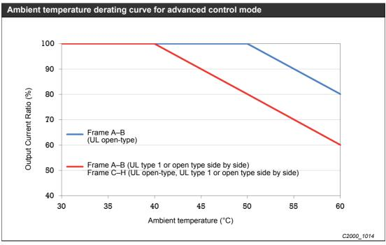
Fig. 12-62: Derating for high ambient temperature
