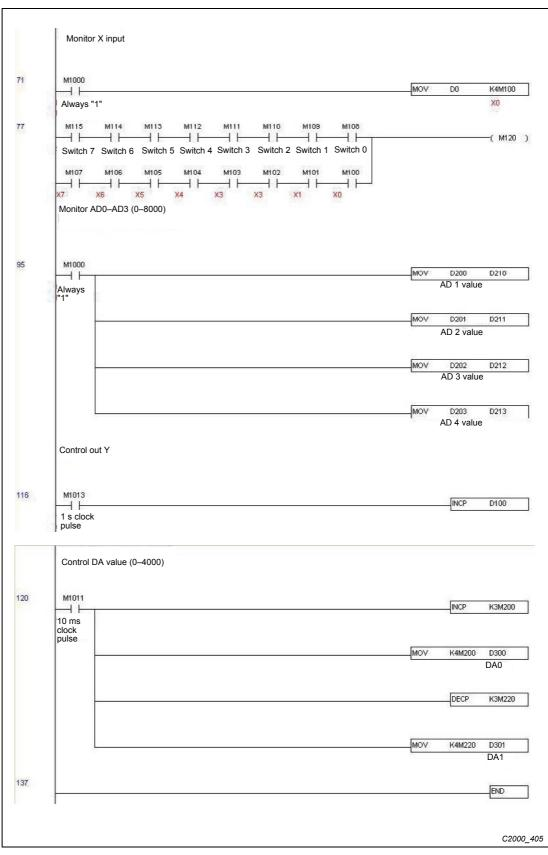
Fig. 16-46: PLC program for communication between C2000 and RTU-485 (2)
