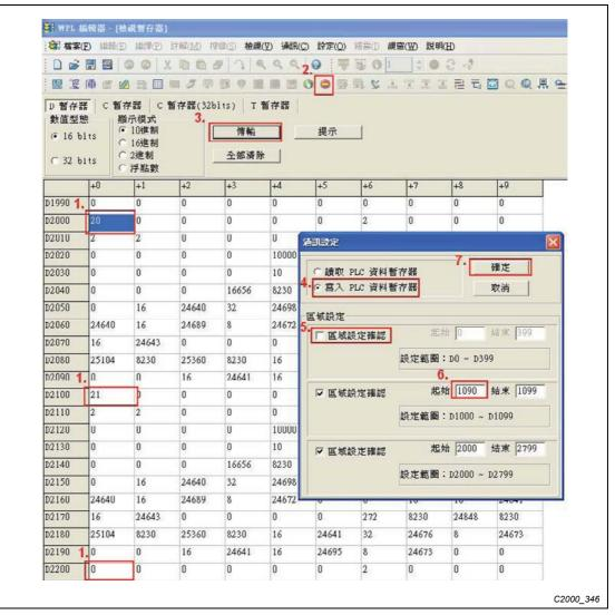
Fig. 16-37: Changing the contents of the special registers for CANopen<sup>®</sup> and download to the PLC
