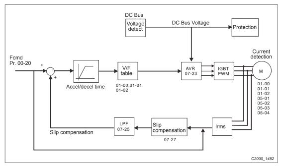
■ When 00-10 = 0, and set Pr. 00-11 to 2, the sensorless vector control diagram is shown as follows:
