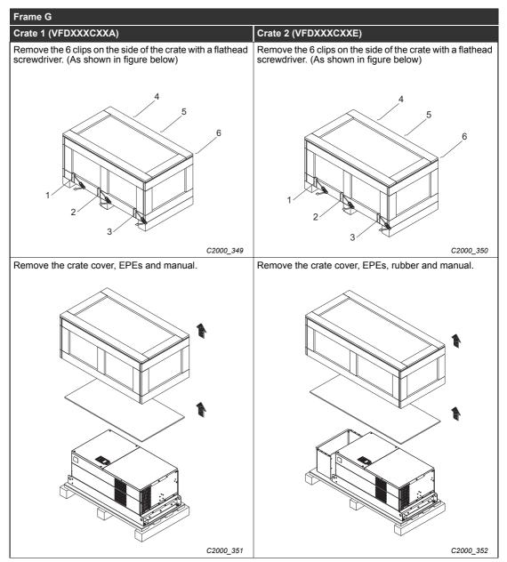
Tab. 2-7: Unpacking inverters of frame size G
