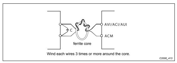
Fig. 6-2: Noise recuction by capacitator and ferrite core
