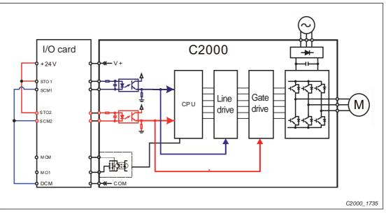
Fig. 20-2: Wiring of STO1/STO2 with +24V and SCM1/SCM2 with DCM
