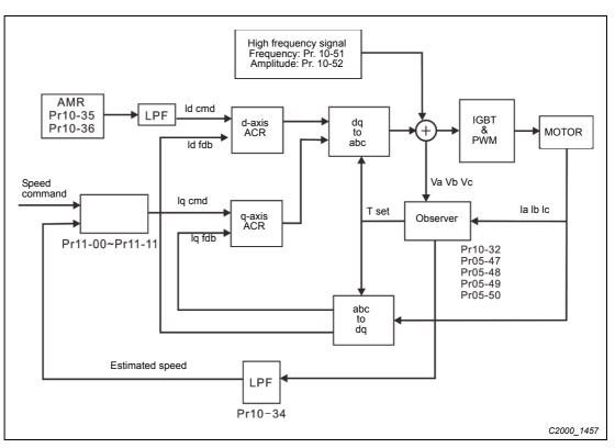
Fig. 12-9: IPM FOC sensorless control diagram
