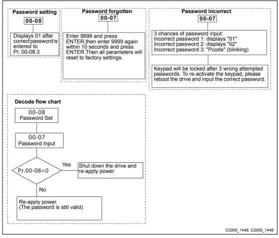
Fig. 12-1: Password decode flow chart
