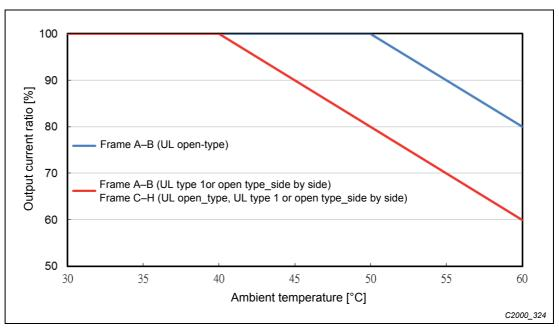
Advanced control ambient temperature derating curve
