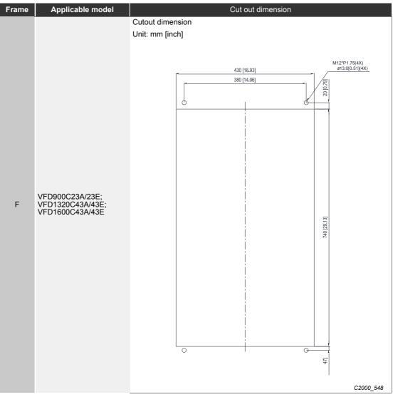
Tab. 7-42: Cut out dimension for plate installation
