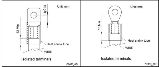
Fig. 5-16: Specification of insulated heat shrink tubing that comply with UL (600 V, YDPU2)
