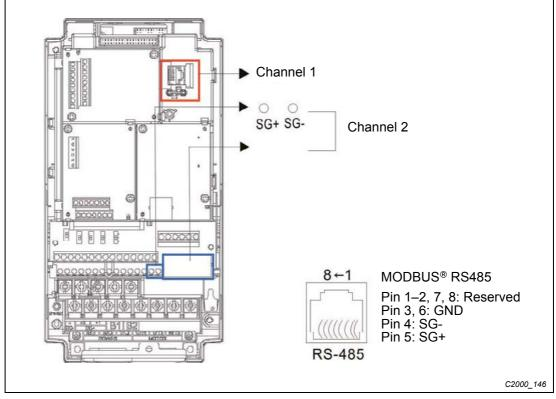
Fig. 16-1: Communication interface of an C2000 inverter
