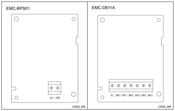
Fig. 8-9: I/O & relay extension card (Slot 3)
