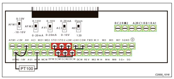
Fig. 12-64: Connection of a PT100 sensor to the I/O control terminal block
