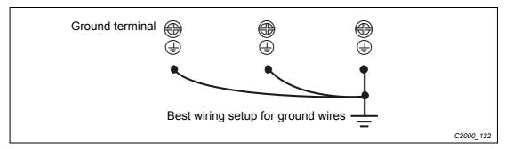
Fig. 1-6: Grounding multiple sets of frequency inverters.
