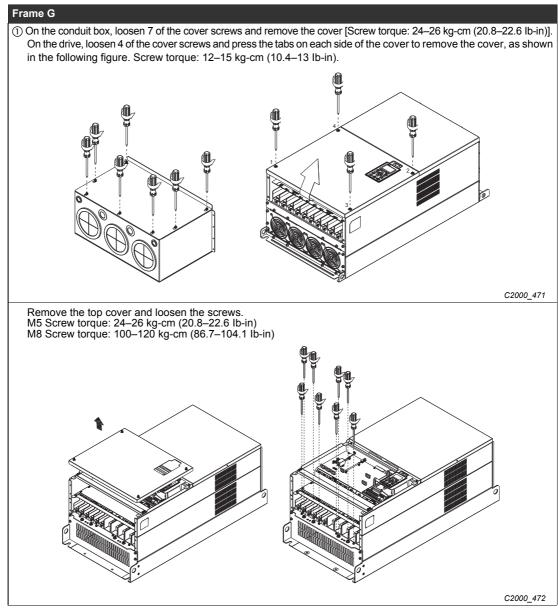
Tab. 7-28: Installation of the conduit box to frame G
