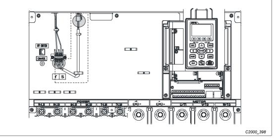
DC-Link testcable for framesize E to H (inclusive common DC-Link or DC supply).
