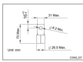
Fig. 5-21: Specification for ring lug
