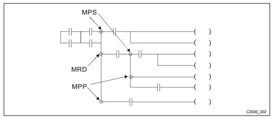
Fig. 16-29: MPS, MRD, and MPP commands
