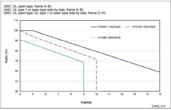
Fig. 12-59: Derating cureve for sensorless control (230 V, ND)
