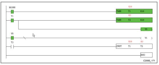
Fig. 16-19: Example for the display of the program in ladder diagram control mode
