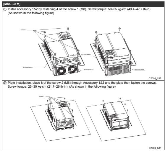
Tab. 7-39: Mounting of accessories and plate installation
