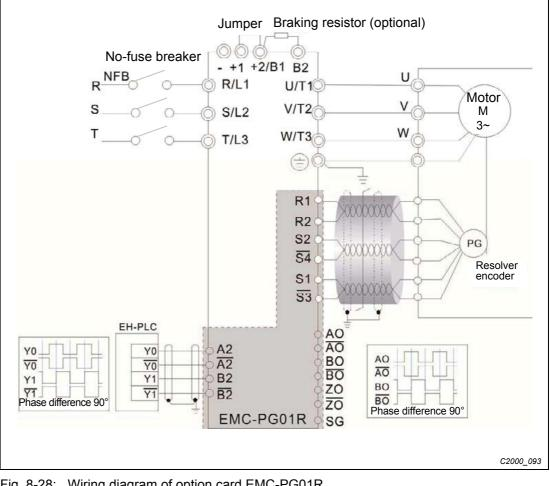
Fig. 8-28: Wiring diagram of option card EMC-PG01R
