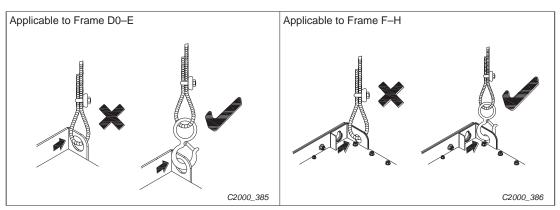
Fig. 2-1: Proper use of the lifting hook
