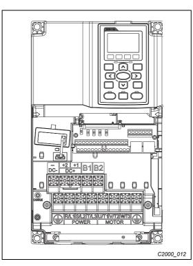
Fig. 5-9: View of frequency inverter frame B
