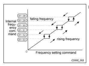
Fig. 12-22: Skip frequency adjustment
