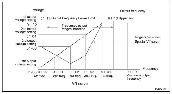
Fig. 12-16:Voltage/frequency ratio
