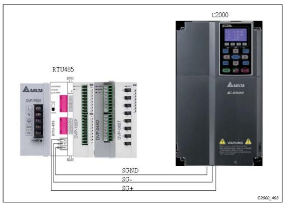
Fig. 16-44: The C2000 communicates with the RTU-485 via the RS485 interface
