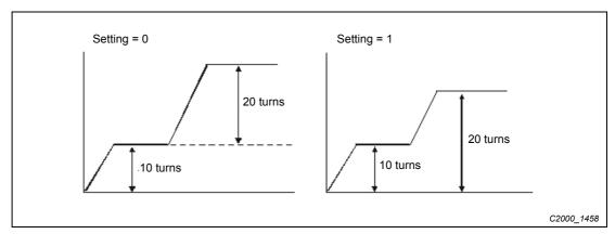
Fig. 12-10:Incremental and absolute type point to point control
