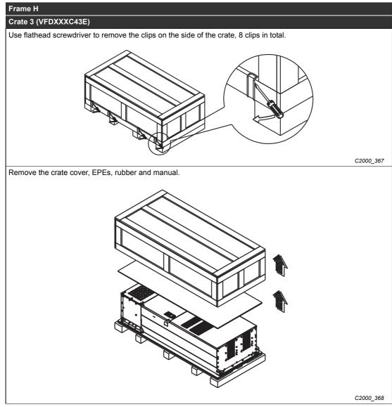
Tab. 2-12: Unpacking inverters of frame size H
