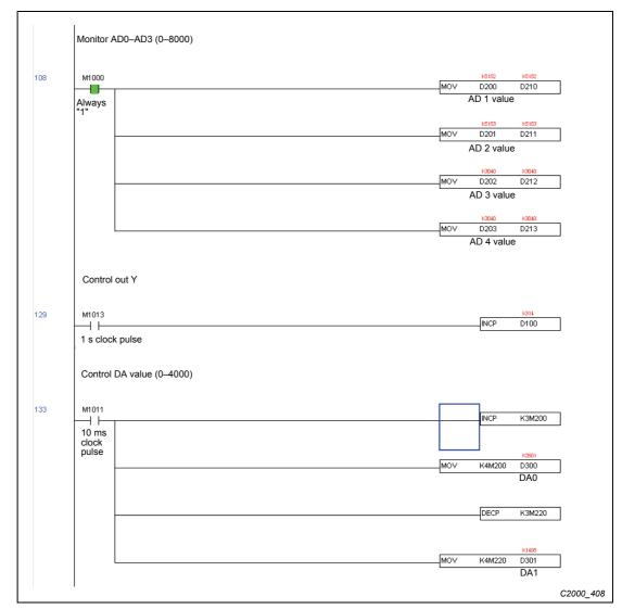
Fig. 16-49: Program part for analog inputs and outputs
