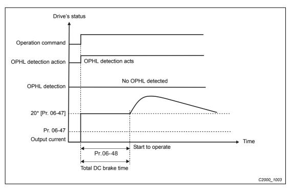
Fig. 12-51: Status 4-1: Pr. 06-48  $\neq$  0, Pr. 07-02 = 0 (No OPHL detected before operation)
