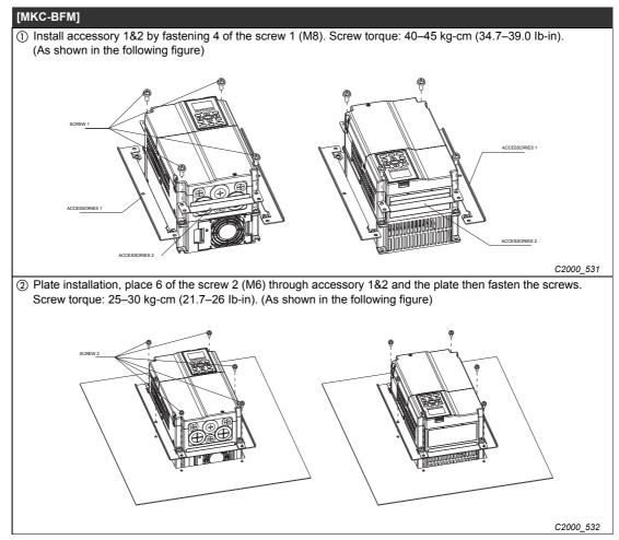
Tab. 7-37: Mounting of accessories and plate installation
