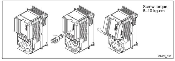
Fig. 8-1: Cover removal and screw tightening torque
