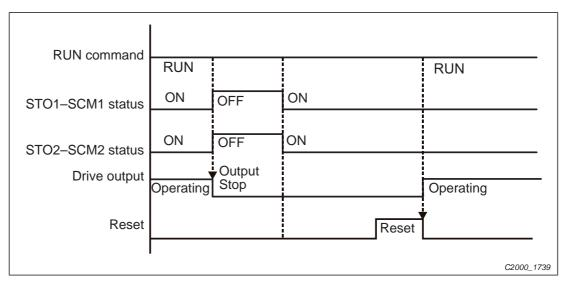
Fig. 20-6: Signal course when enabling STO1-SCM1, STO2-SCM2 with Pr. 02-35 = 1
