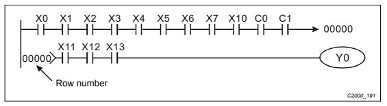
Fig. 16-21: The whole row contains more than 11 contacts and is therefore divided.
