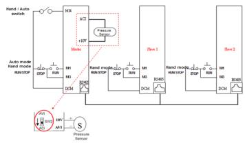
Wiring of the pressure sensor:
