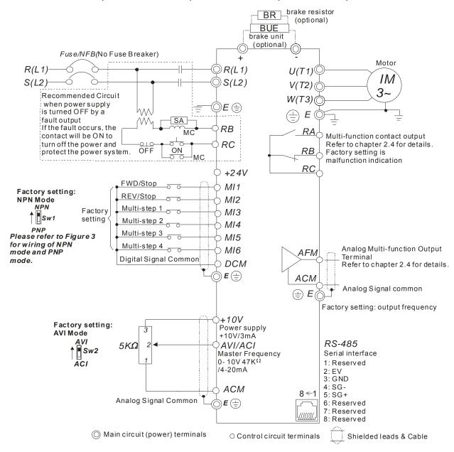
$Figure\ 2\ for\ models\ of\ VFD-EL\ Series\\ VFD002EL23A,\ VFD004EL23A/43A,\ VFD007EL23A/43A,\ VFD015EL23A/43A,$
