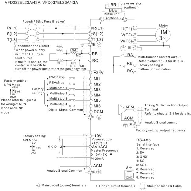
Figure 3 Wiring for NPN mode and PNP mode
