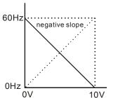
Pr.01.00=60Hz--Max. output Freq. Potentiometer Pr.04.00 =100%--Bias adjustment
