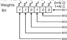
The setting value =  $bit5x2^5 + bit4x2^4 + bit2x2^2$ =  $1x2^5 + 1x2^4 + 1x2^2$ = 32 + 16 + 4 = 52Setting 04.09
