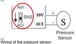
Connect pressure sensor to +10V and AVI, then switch the SW2 switch to ACI
