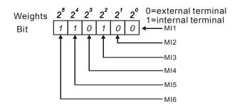
04.28# Internal Terminal StatusUnit: 1Settings0 to 4095Factory Setting: 0
