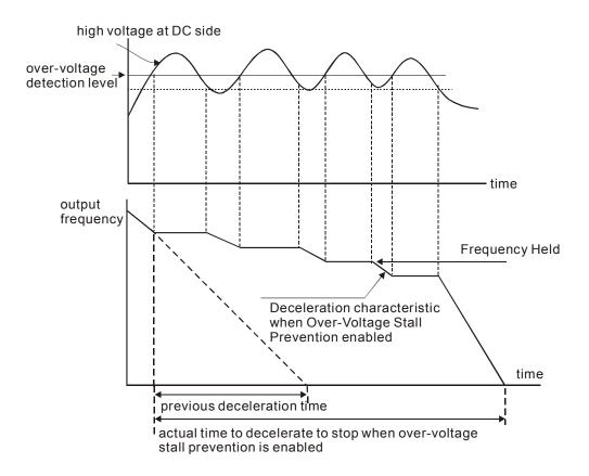
Over-Voltage Stall Prevention must be disabled (Pr.06.00=0) when a brake unit or brake resistor is used.
