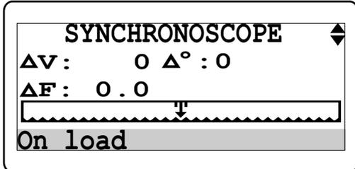
This page is for observing level differences between generator and mains voltage, frequency and phase angle. When an uninterrupted transfer is in progress, synchronoscope page will be shown automatically.
