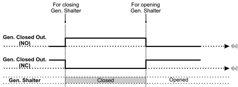
**1- User Configured:** Mains and Gen breakers have only close drives, when want to breaker close, close breaker output on and after 1 sec. open breaker output on and after breaker close pulse time open breaker output will off. When want to breaker open close breaker output and open breaker output will off.
